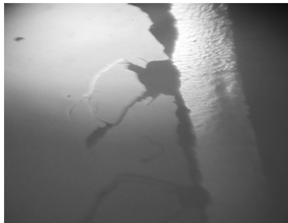
Fig. 5. Damage trace of filament in switch sample triggered 1500 times.
