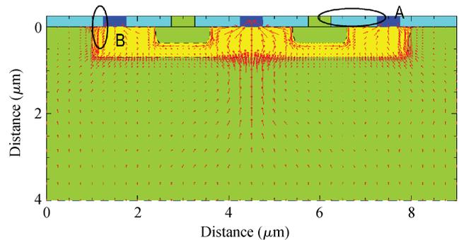
Fig. 6. Distributions of the current density at 5 ns.
