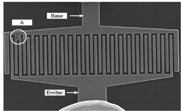
Fig. 1. SEM image of a molten region between the emitter and base.
