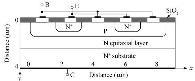
Fig. 3. Structural sketch map of a multifinger BJT.
