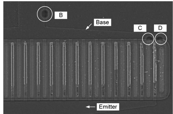
Fig. 2. SEM image of the ESD failure of the BJT after removing the passivation and metal layers.
