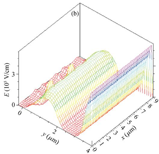
Fig. 5. Distributions of electric field under ESD stress at different times. (a) Before avalanche breakdown at 5 ns. (b) After avalanche breakdown at 15 ns.
