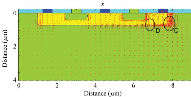
Fig. 8. Nonuniform distributions of the current density at 20 ns.
