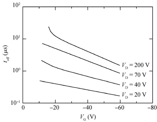
Fig. 2. Dependence of switching-off time  $t_{off}$  on  $V_G$  and  $V_D$ .
