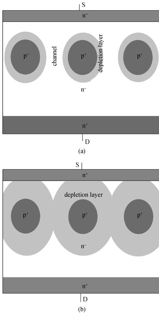
Fig. 4. Profile of the depletion layer at (a) forwardly conducting state and (b) forwardly blocking state.
