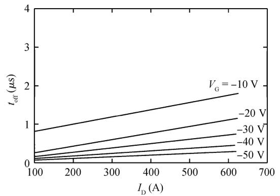
Fig. 3. Dependence of switching-off time on  $I_D$  and  $V_G$ .
