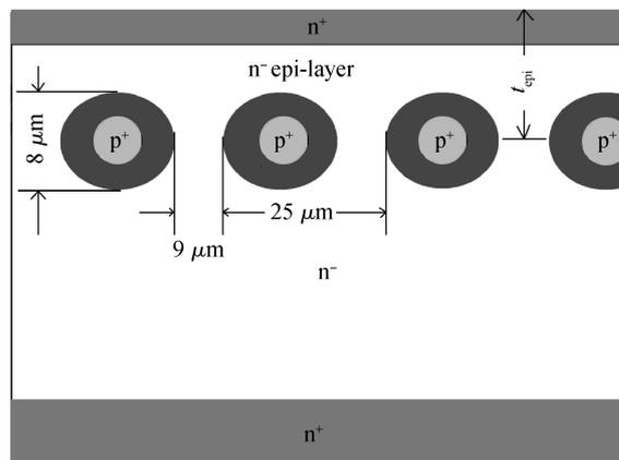
Fig. 1. Cross-section of a segment of BSIT with buried gate structure.
