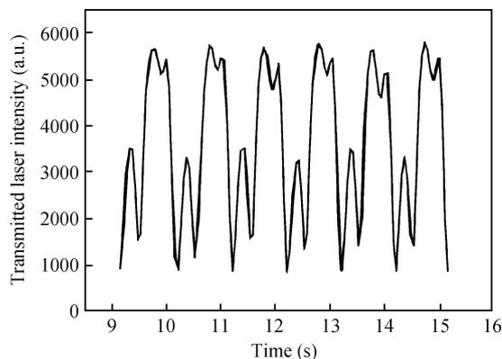
Fig. 2. Time evolution of the relative transmitted intensity of the probe beam for sample 1 when an AC voltage with a frequency of 0.5 Hz is applied.
