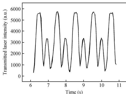
Fig. 3. Time evolution of the relative transmitted intensity of the probe beam for sample 2 when an AC voltage with a frequency of 0.5 Hz is applied.
