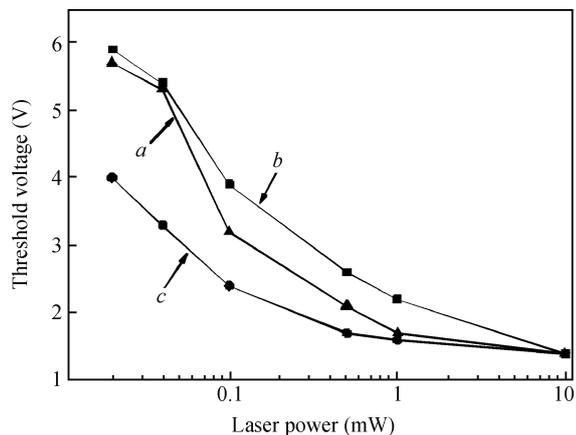
Fig. 1. Threshold voltages in different configurations. (a) Sample 1. (b) Sample 2 with forward voltage. (c) Sample 2 with reverse voltage.
