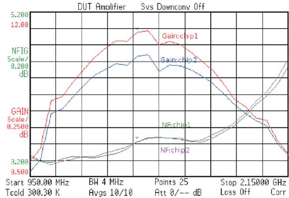
Fig. 8. Measured noise figure and power gain of LNA loop out versus frequency.
