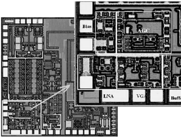
Fig. 6. Die photograph of the wideband amplifier.
