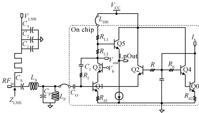
Fig. 2. Simplified schematic of a wideband LNA.
