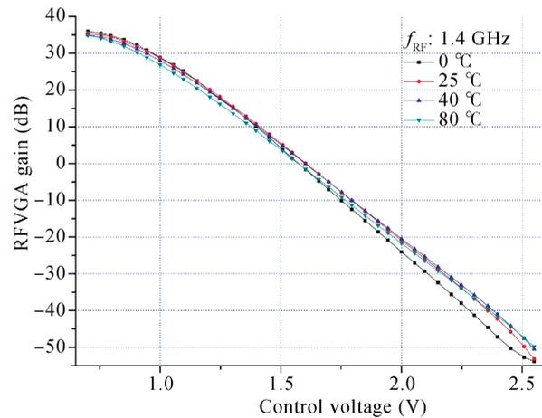
Fig. 9. Measured VGA gain versus control voltage over temperature.
