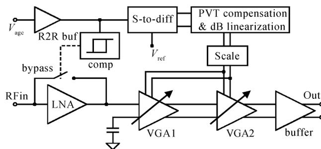
Fig. 1. Block diagram of the wideband amplifier
