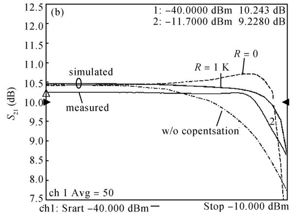
Fig. 3. Measured and simulated LNA distortion compensation. (a) LNA bias current versus RF input. (b) LNA loop output power gain versus RF input.
