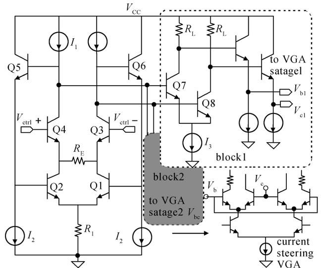
Fig. 5. Simplified schematic of the scaling circuit.
