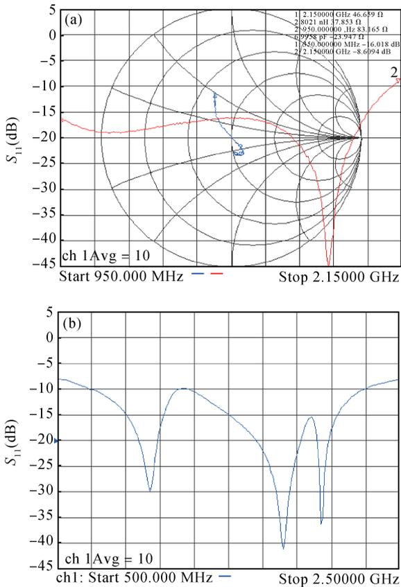
Fig. 7. Measured wideband LNA input matching. (a) Without the LNB transmission line. (b) With the LNB transmission line.
