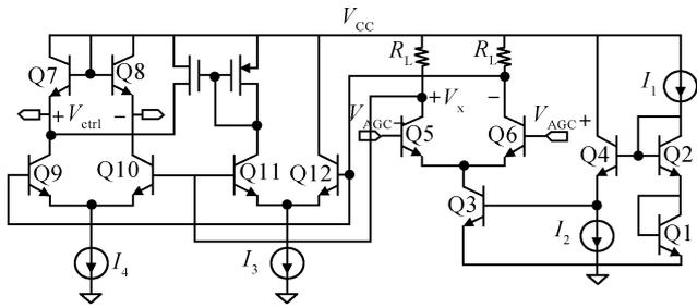
Fig. 4. Simplified schematic of a PVT compensation and dB linearization circuit.
