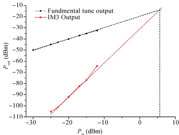
Fig. 10. Measured two-tune test of the wideband amplifier at low gain.
