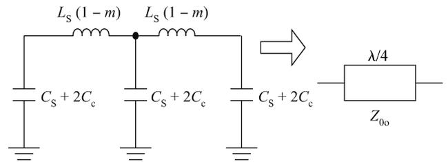
Fig. 4. Lumped equivalent circuit for an odd mode circuit of  $\lambda/4$  coupled line.
