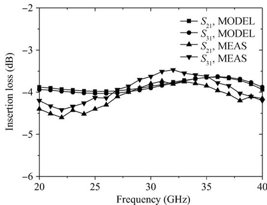
Fig. 10. Measured and simulated insertion losses of the balun.
