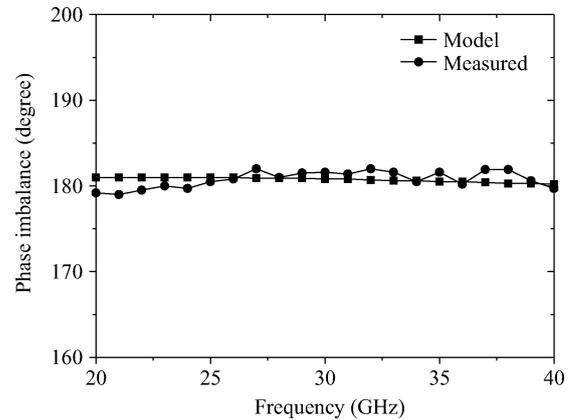
Fig. 11. Measured and simulated phase imbalance of the balun.
