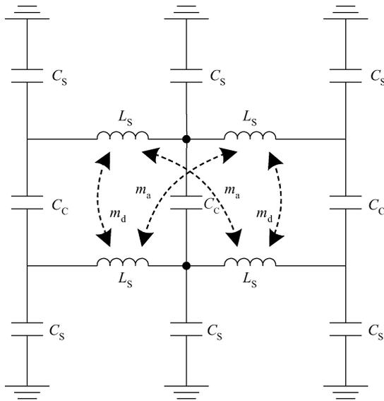
Fig. 2. Lumped element equivalent circuit of a coupled line.
