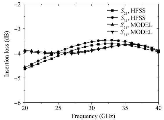
Fig. 7. Simulated insertion losses of the balun.
