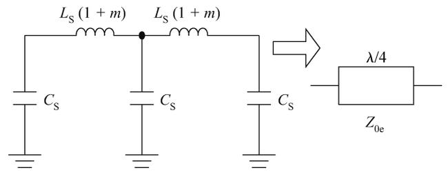
Fig. 3. Lumped equivalent circuit for even mode circuit of a  $\lambda/4$  coupled line.
