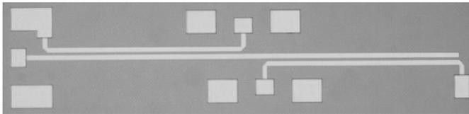
Fig. 9. Microphotograph of fabricated balun.
