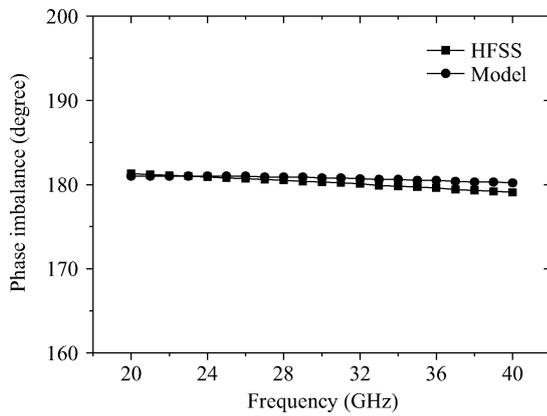
Fig. 8. Simulated phase imbalance of the balun.
