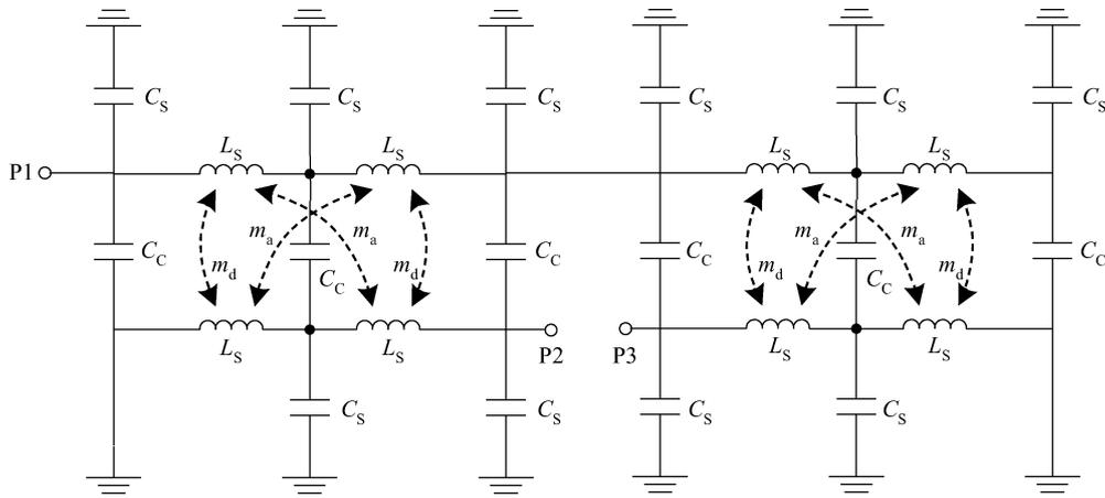
Fig. 5. Lumped element equivalent circuit of a Marchand balun.
