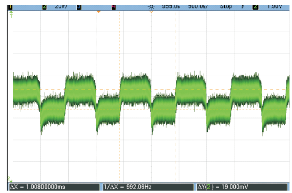
(a) Load transient response
