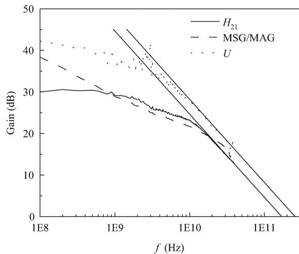
Fig. 3.  $H_{21}$ , MSG/MAG and  $U$  of the DHBT with emitter area of  $1 \times 15 \mu\text{m}^2$  at  $V_{CE} = 2.0 \text{ V}$  and  $I_C = 22 \text{ mA}$ .
