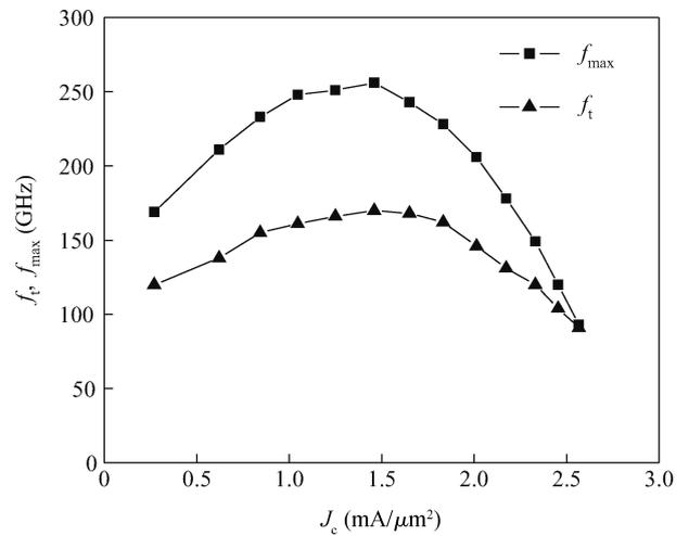
Fig. 4. Variation of  $f_t$  and  $f_{\text{max}}$  versus  $J_c$  for the DHBT with emitter area of  $1 \times 15 \mu\text{m}^2$  at  $V_{CE} = 2.0 \text{ V}$ .
