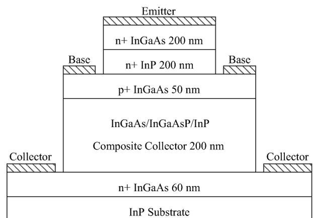
Fig. 1. Layer structure of the InGaAs/InP DHBT.
