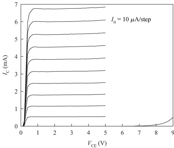
Fig. 2. Typical common-emitter  $I-V$  curves of a  $1 \times 15 \mu\text{m}^2$  InP DHBT device.
