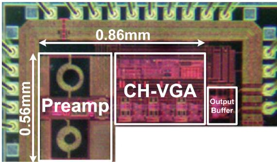
Fig. 9. Die microphotograph of the proposed VGA.
