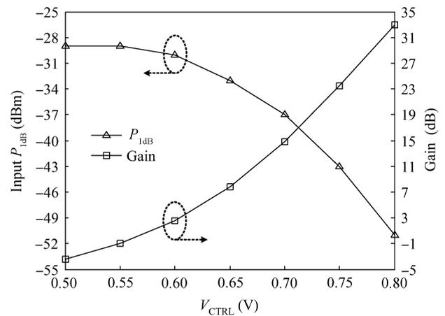
Fig. 12. Measured  $P_{1dB}$  and gain versus  $V_{CTRL}$  @ 1.9 GHz.
