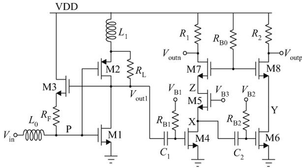
Fig. 2. Simplified schematic of the pre-amplifier.
