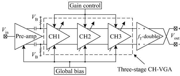
Fig. 1. Block diagram of the proposed VGA architecture.
