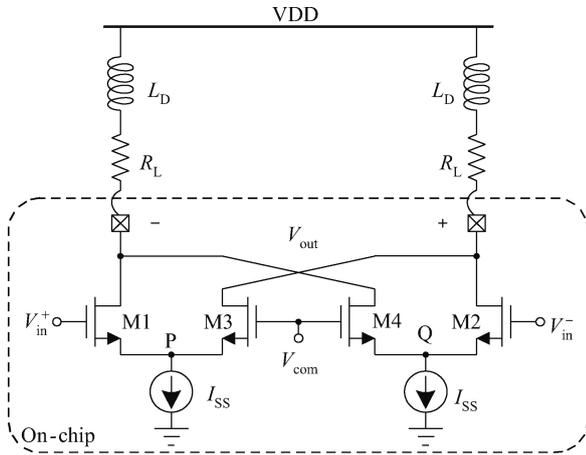
Fig. 8.  $f_T$ -doubler output buffer.
