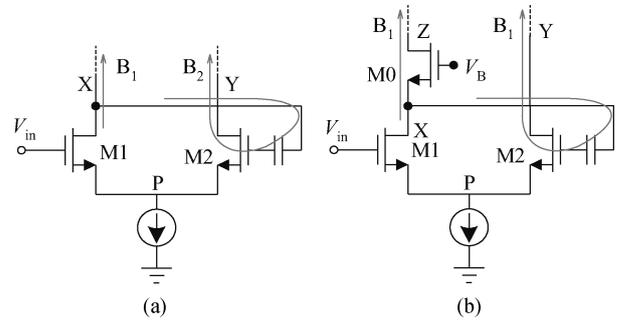
Fig. 3. Comparison of (a) conventional and (b) proposed active balun circuits.
