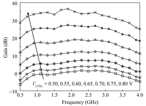
Fig. 11. Measured frequency response under different control voltages.
