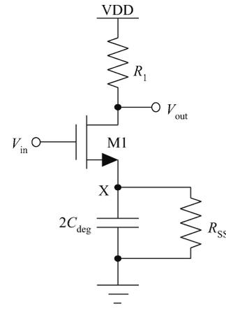
Fig. 6. Equivalent half-circuit of Gm1 for DCOC.
