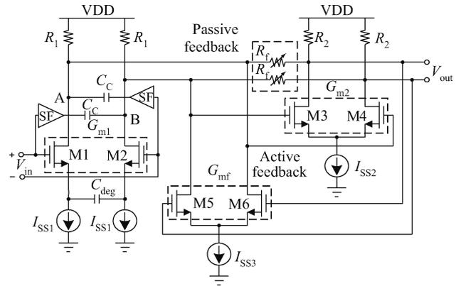
Fig. 5. Realization of the proposed variable gain Cherry–Hooper amplifier.
