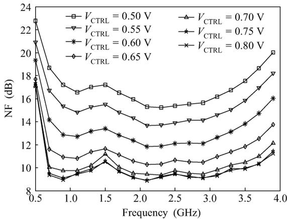
Fig. 13. Measured noise figure response versus various control voltage  $V_{\text{CTRL}}$ .
