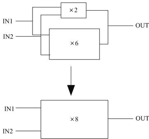
Fig. 1. A parallel cell realization example.
