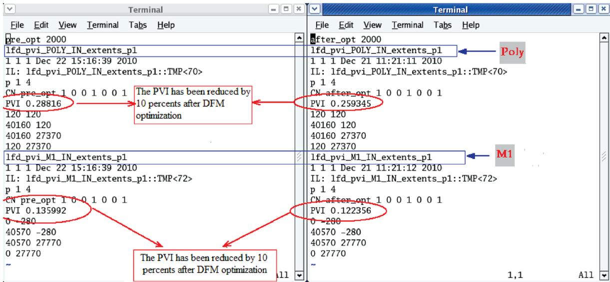
Fig. 9. Result of the PVI test for standard cells.
