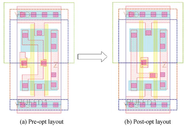
Fig. 2. Layout of buffer cell.
