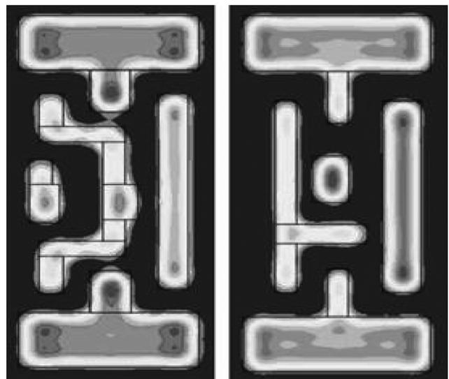
Fig. 3. Metal of buffer after optical simulation.
