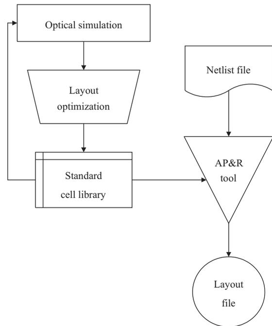
Fig. 5. Design flow of standard cell library which includes the optical simulation stage.
