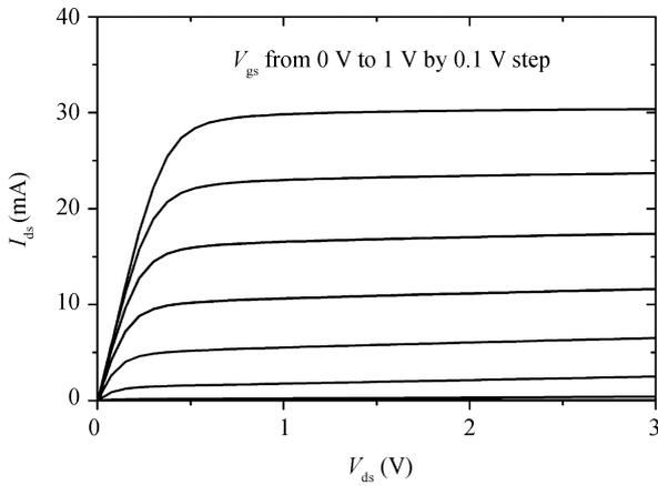
Fig. 2. DC-I-V characteristics of the FET.
