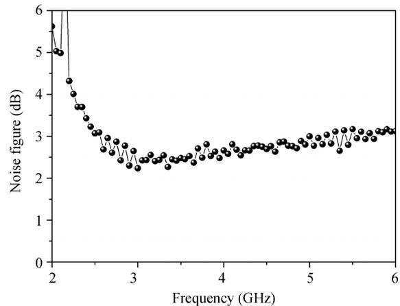
Fig. 9. Measured noise figure of the LNA.
