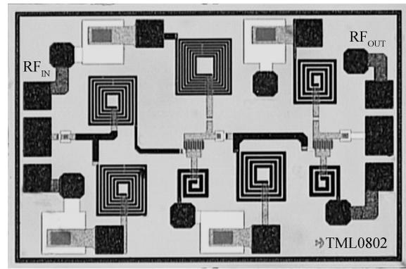
Fig. 7. Chip photograph of the LNA.
