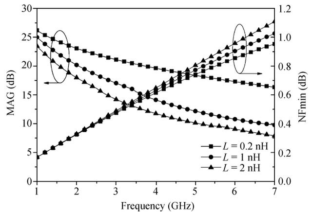
Fig. 4. Simulation of MAG/MSG and  $NF_{min}$  of the first stage with various source degeneration inductor values.
