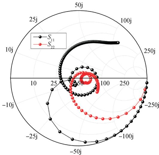
Fig. 6. Simulation of input/output  $S$ -parameters of the LNA.
