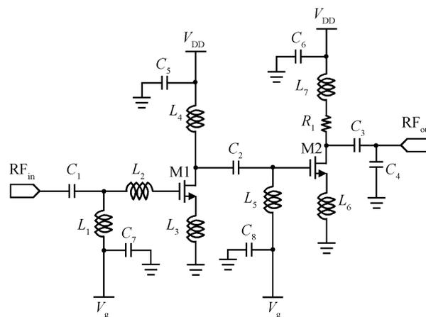
Fig. 1. Schematic of the proposed LNA.
