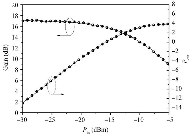
Fig. 10. Power performance of the LNA at 4 GHz.
