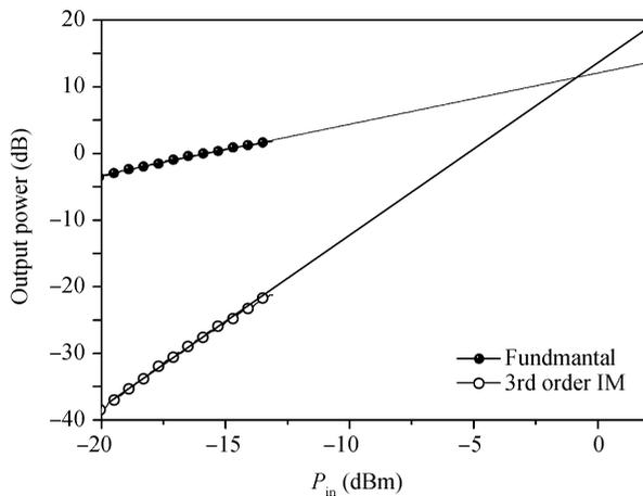
Fig. 11. Third-order intercept point of the LNA at 4 GHz.
