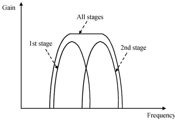
Fig. 5. Gain profiles of the two-stage LNA.
