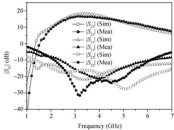
Fig. 8. Simulated and measured small signal gain and return losses of the LNA.
