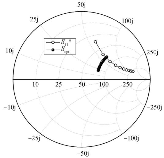
Fig. 3.  $S_{opt}$  and conjugate of  $S_{11}$  versus source degeneration inductors.
