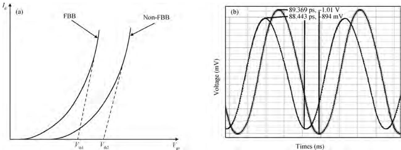
Fig. 3. Effect of FBB technique. (a) RFMOS  $I-V$  curve. (b) LC-VCO oscillation amplitude.
