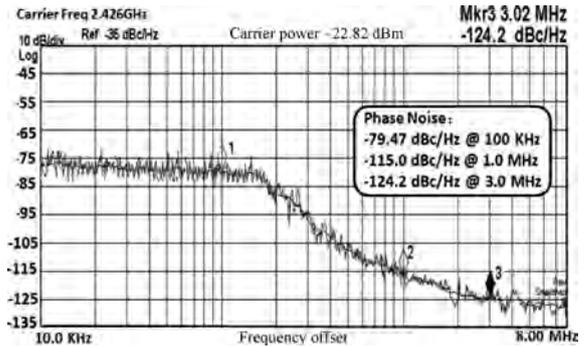
Fig. 21. The measured phase noise of the synthesizer @ 2.426 GHz.
