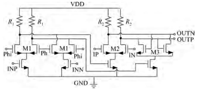
Fig. 7. Phase-switchable level-sensitive (PSLS) latches.
