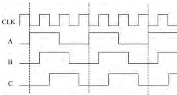
Fig. 8. Divide-by-3 timing diagram.
