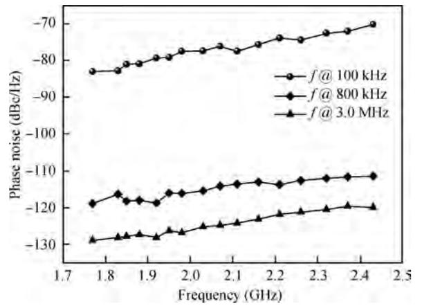
Fig. 20. The measured phase noise of Freq1 (1.75–2.5 GHz).
