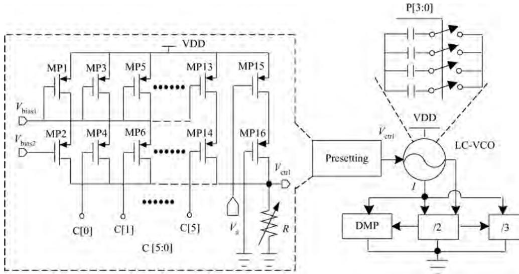
Fig. 4. LC-VCO with presetting module.
