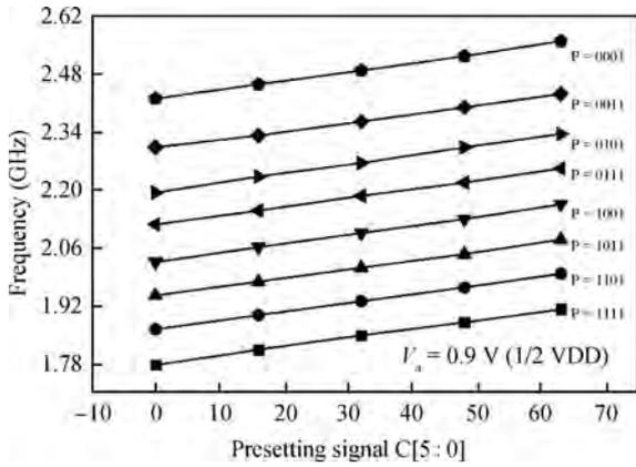
Fig. 17. Frequency versus presetting signal C[5 : 0] with different values P[3 : 0].
