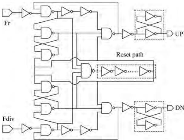
Fig. 13. Schematic of the dead-zone-free PFD.
