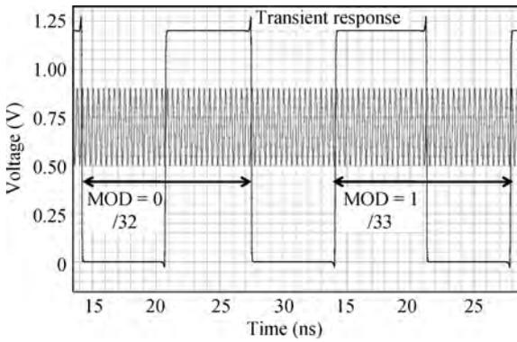
Fig. 12. Transient simulation of the DMP @ 2.4 GHz.
