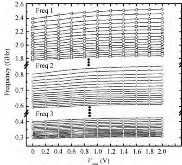
Fig. 16. The measured three frequency bands of the synthesizer.
