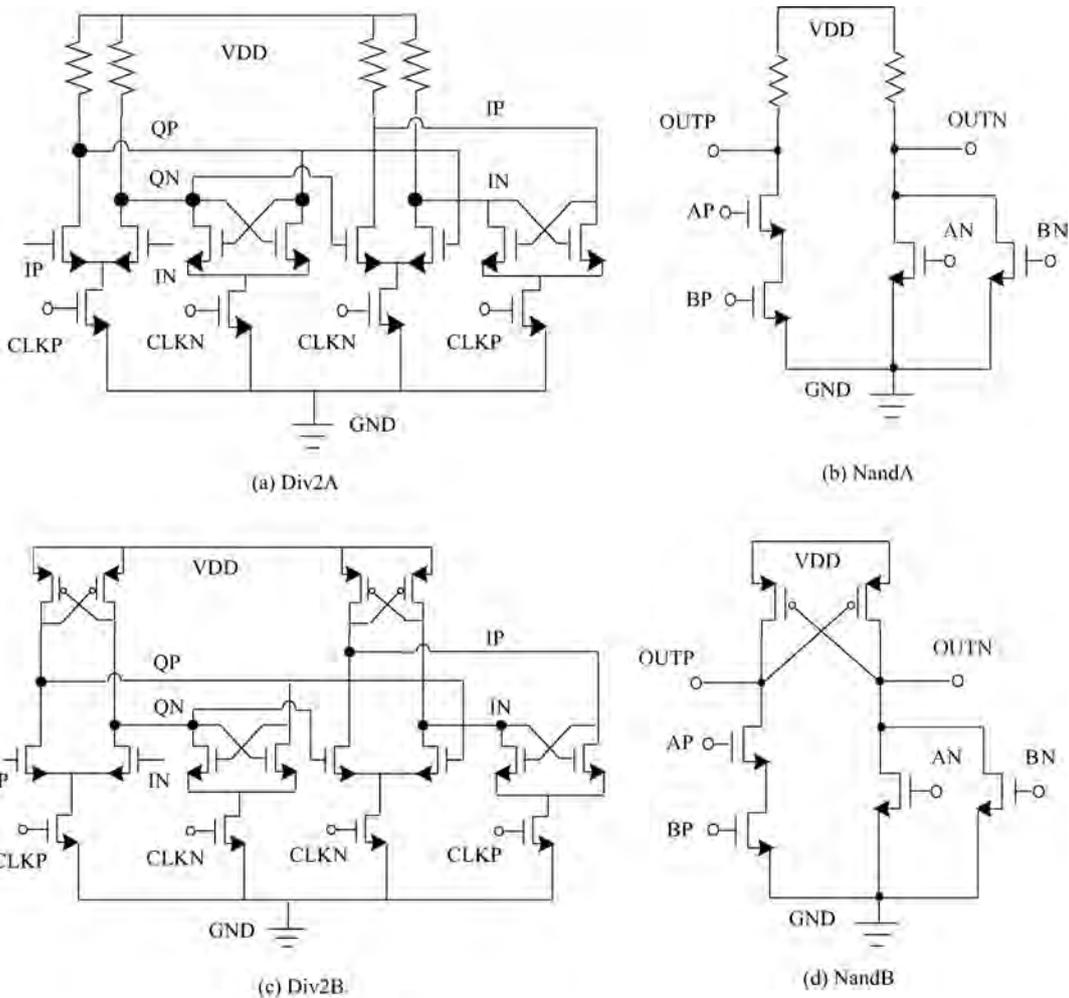
Fig. 11. Different dividers and NAND gates in DMP.
