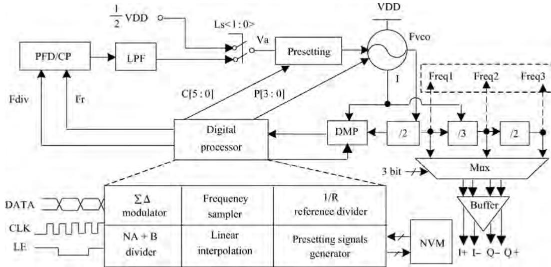
Fig. 1. Architecture of the proposed frequency synthesizer.
