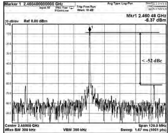
Fig. 22. The measured spectrum of the synthesizer @ 2.460 GHz.
