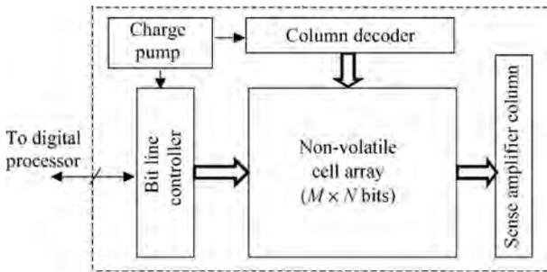
Fig. 5. Architecture of the NVM.
