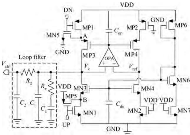
Fig. 14. Schematic of charge pump and LPF.
