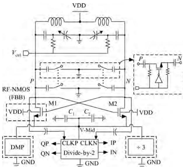
Fig. 2. Current reusing LC-VCO and stacked modules.
