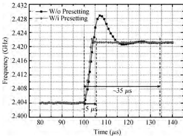
Fig. 18. Typical settling time of the synthesizer.
