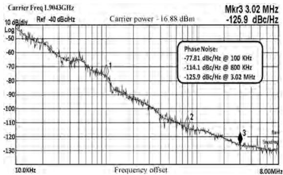
Fig. 19. Phase noise of the Freq1 @ 1.9 GHz.
