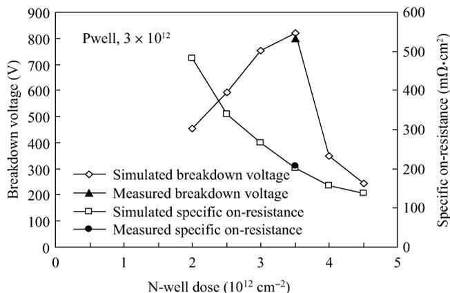
Fig. 4. Off-state breakdown voltage and specific on-resistance as a function of N-well dose with P-well dope of  $3 \times 10^{12} \text{ cm}^{-2}$  for 700 V double RESURF LDMOS.
