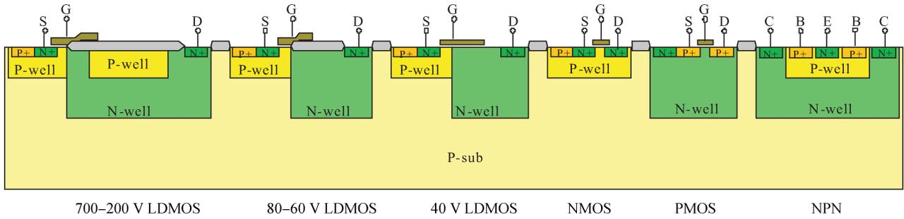
Fig. 1. Schematic cross-sectional view of 700 V BCD technology.
