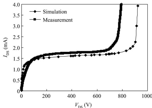
Fig. 7. Drain current characteristics for 700 V nJFET.
