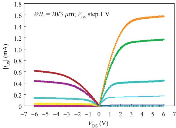
Fig. 8. Drain current characteristics for low voltage CMOS.
