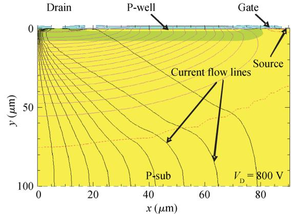
Fig. 2. The simulated potential contours of 700 V double RESURF LDMOS.
