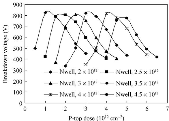
Fig. 3. The simulated off-state breakdown voltage as a function of P-top dose with different N-well dose for 700 V double RESURF LD-MOS.
