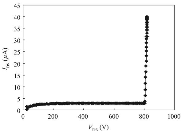
Fig. 5. The measured off-state breakdown characteristics of 700 V double RESURF LDMOS.
