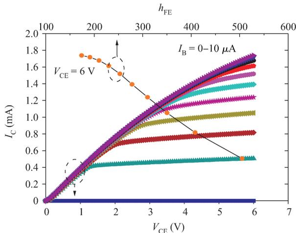
Fig. 9.  $I_C$ - $V_{CE}$  and  $h_{FE}$ - $I_C$  characteristics for NPN.
