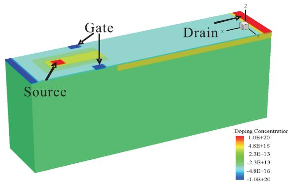
Fig. 6. The simulated structure for 700 V nJFET by ISE.
