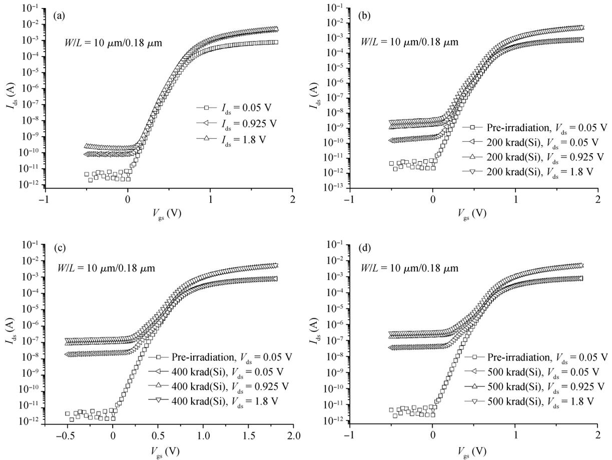
Fig. 3. Influence of drain bias on the pre-irradiated and irradiated transistors. (a) Pre-irradiation, (b) 200, (c) 400 and (d) 500 krad(Si).
