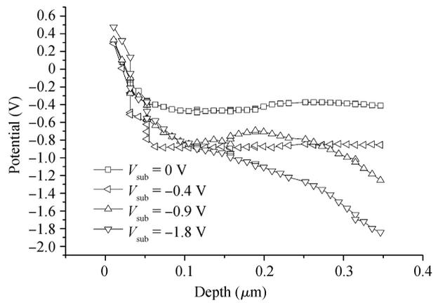
Fig. 8. Potential profile along the STI depth as a function of substrate bias.
