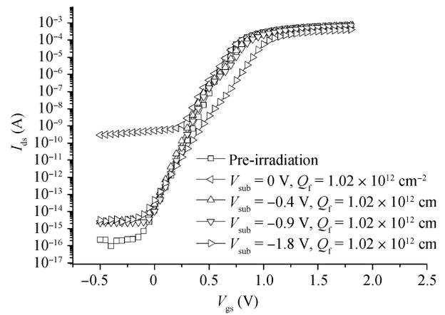
Fig. 7. Simulation results with uniform charge distribution along the STI interface for different substrate biases.
