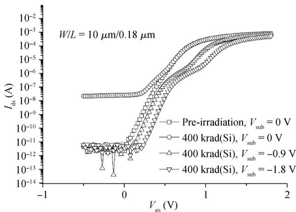
Fig. 6. Influence of substrate bias on the 400 krad(Si) irradiated transistor, compared with the pre-irradiated  $V_{sub} = 0$  V.
