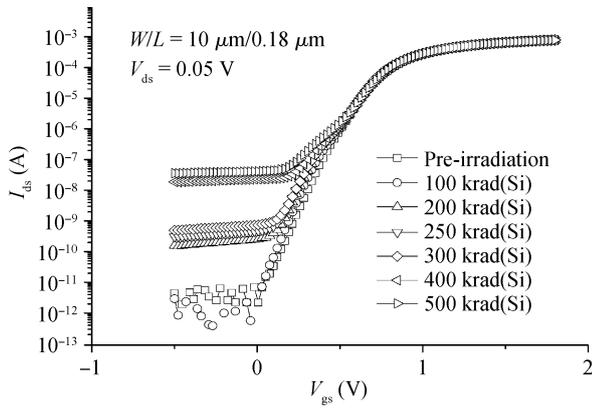
Fig. 1.  $I_{ds}$ - $V_{gs}$  characteristics as a function of dose for the irradiated transistors with  $W/L = 10/0.18 \mu\text{m}$ .
