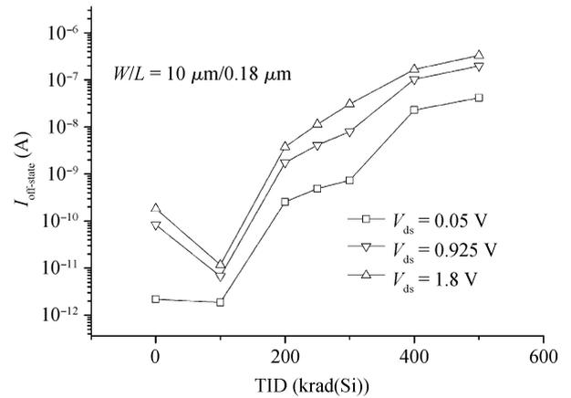
Fig. 4. Evolution of leakage current with TID for drain biases of 0.05, 0.925 and 1.8 V.
