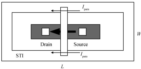
Fig. 2. Drain-to-source leakage path in an NMOSFET.
