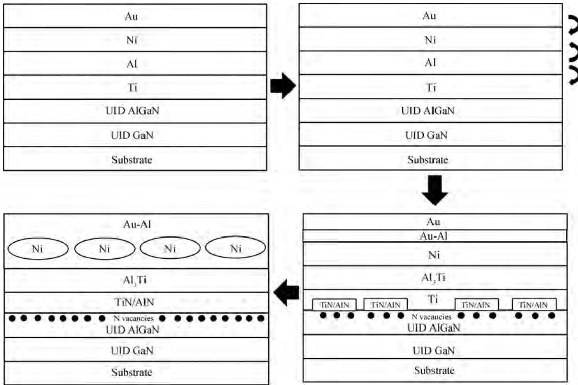
Fig. 5. The metal alloy process in rapid thermal annealing.
