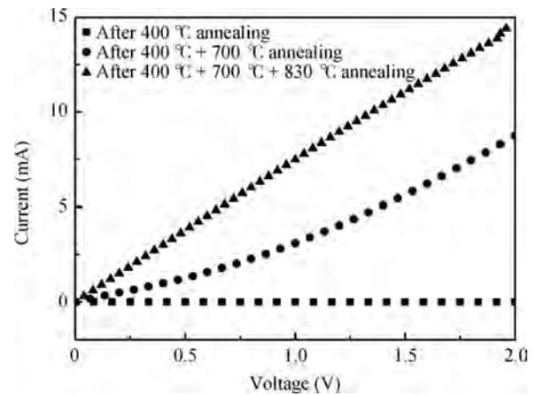
Fig. 8. The current–voltage characteristics of the ohmic contact after each step during multi-steps.
