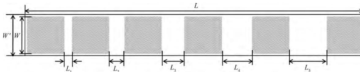
Fig. 2. Image of the TLM test pattern.  $W = 100 \mu\text{m}$ ;  $W' = 110 \mu\text{m}$ ;  $L = 910 \mu\text{m}$ ;  $L_1 = 20 \mu\text{m}$ ;  $L_2 = 40 \mu\text{m}$ ;  $L_3 = 60 \mu\text{m}$ ;  $L_4 = 80 \mu\text{m}$ ;  $L_5 = 100 \mu\text{m}$ .
