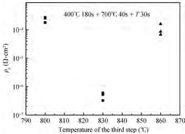
Fig. 7. Dependence of  $\rho_c$  on the annealing temperature of the third step.
