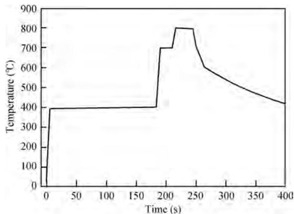
Fig. 1. The process of multi-step annealing.
