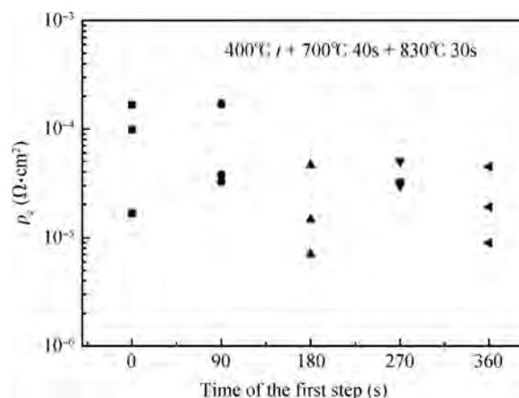
Fig. 3. Dependence of  $\rho_c$  on the annealing time of the first step.
