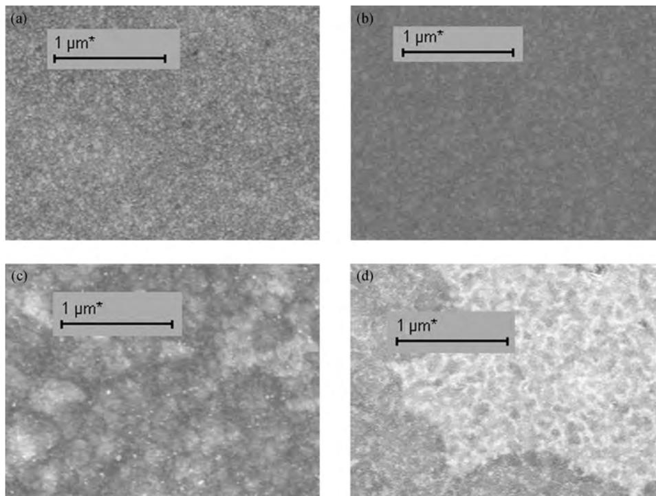
Fig. 9. The surface morphology of the ohmic contact after each step during multi-steps: (a) as-deposited, (b) after 400 °C, (c) after 400 °C + 700 °C, (d) after 400 °C + 700 °C + 830 °C.
