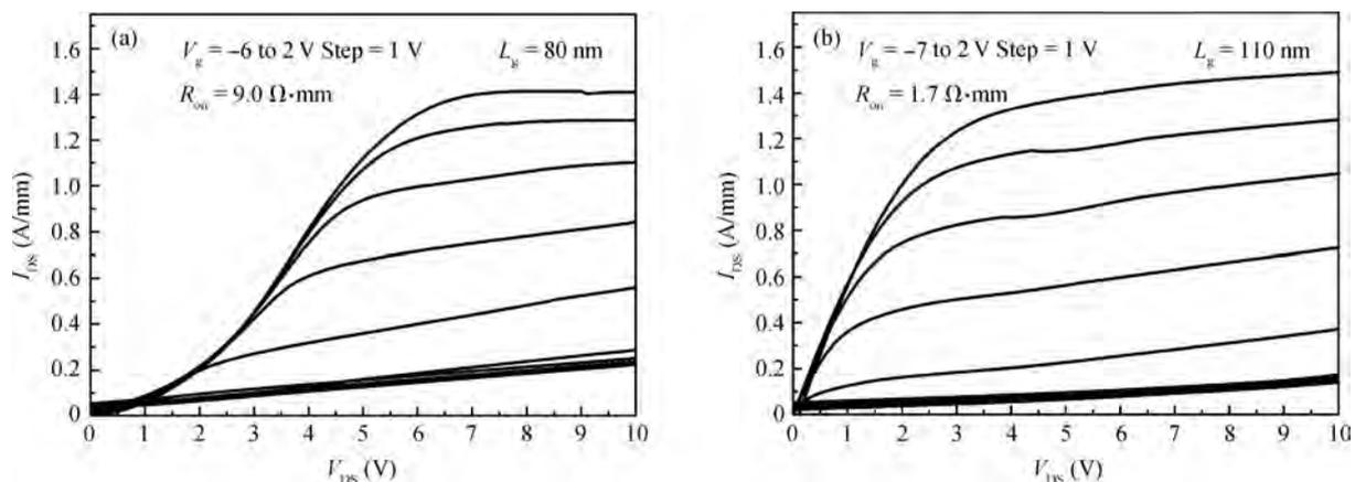
Fig. 10.  $I$ - $V$  characteristics of the AlGaIn/GaN HEMT devices. (a) Annealed at 835 °C for 30 s. (b) Annealed at 400 °C 3 min + 700 °C 40 s + 830 °C 30 s.
