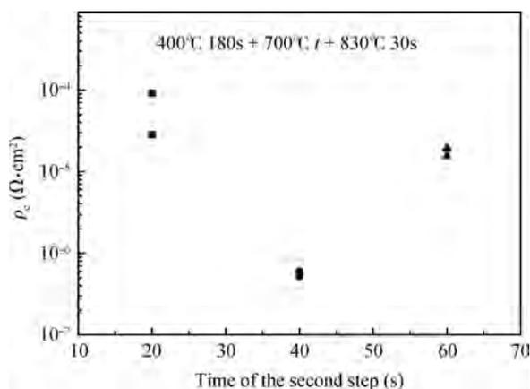
Fig. 4. Dependence of  $\rho_c$  on the annealing time of the second step.
