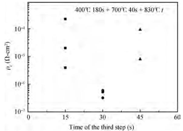
Fig. 6. Dependence of  $\rho_c$  on the annealing time of the third step.
