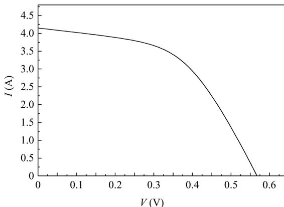
Fig. 3.  $I-V$  curve of the black Si solar cell.
