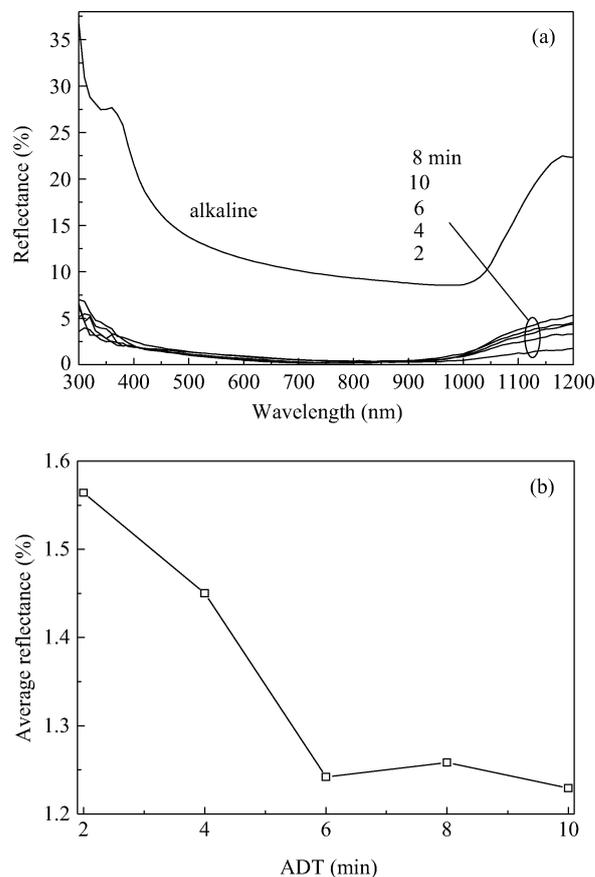
Fig. 2. (a) Reflectivity of the sample surfaces at various ADT. (b) ADT-dependence on the average reflectivity in the 300–1200 nm range.
