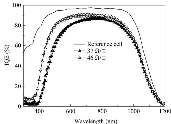
Fig. 5. IQE measurements of black Si solar cells.
