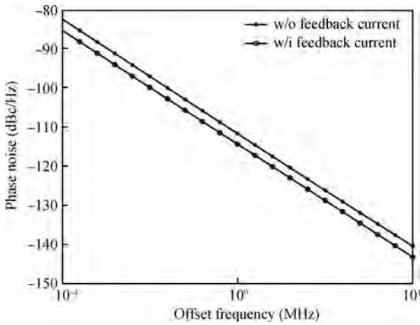
Fig. 3. Simulated phase noise at 3.27-GHz with and without a feedback current source.
