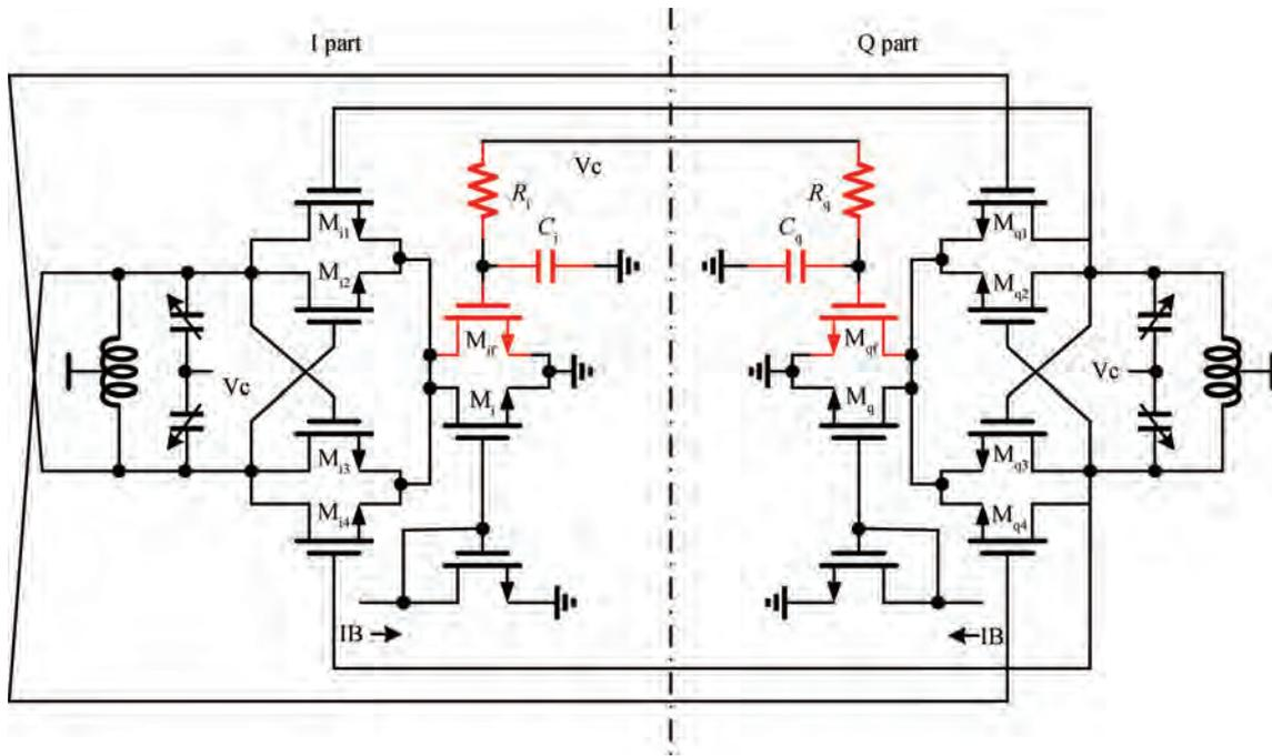
Fig. 1. Proposed QVCO with feedback current source.
