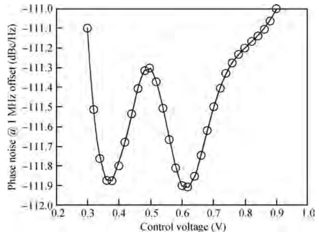
Fig. 9. Measured phase noise at 1 MHz offset versus control voltage.
