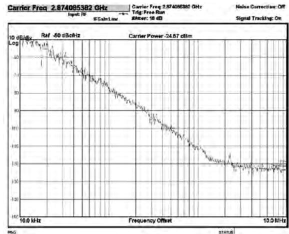
Fig. 8. Measured phase noise at 2.874 GHz.
