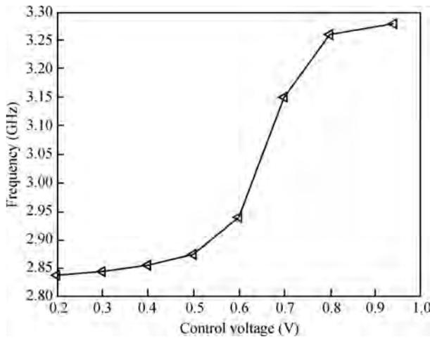
Fig. 6. Measured tuning range of the proposed QVCO.
