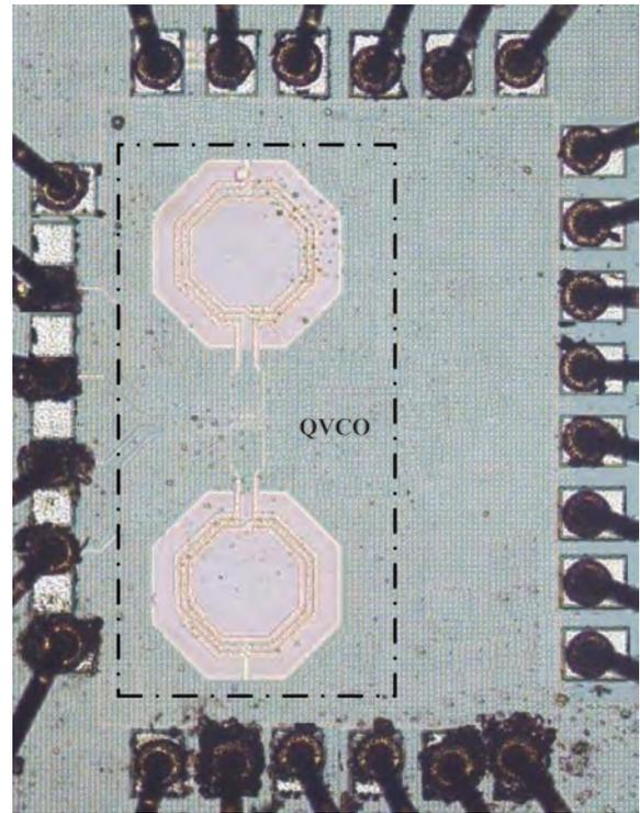
Fig. 5. Chip micrograph of the proposed QVCO.
