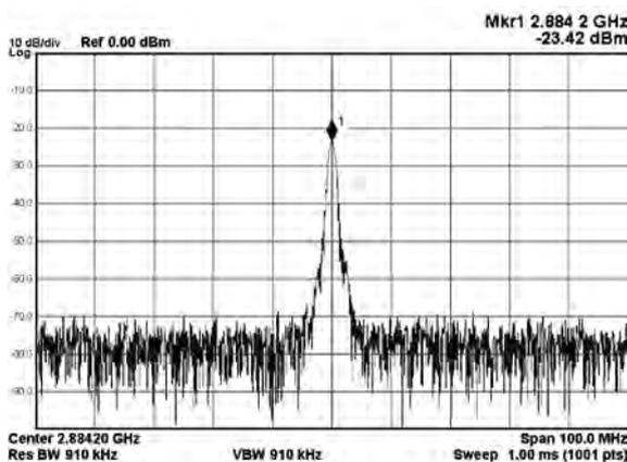
Fig. 7. Measured power spectrum density of the proposed QVCO.
