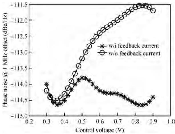
Fig. 4. Simulated phase noise over the control voltage range with and without a feedback current source.
