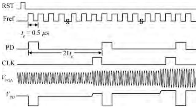
Fig. 10. Timing and signal waveforms of the AGC.
