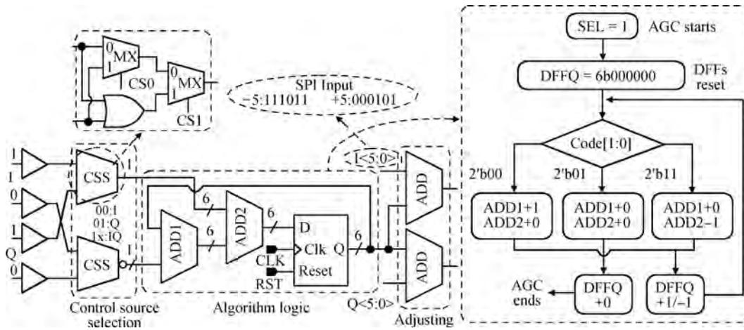
Fig. 9. Block and flowchart of the AGC algorithm logic.
