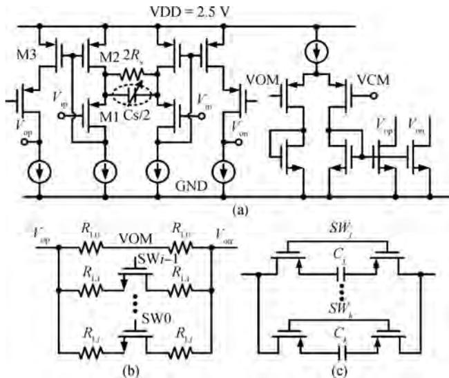
Fig. 3. The improved source degenerated amplifier. (a) Main amplifier with CMFB. (b) Load resistors  $R_L$  array. (c) Source degenerated capacitor  $C_s$  array.
