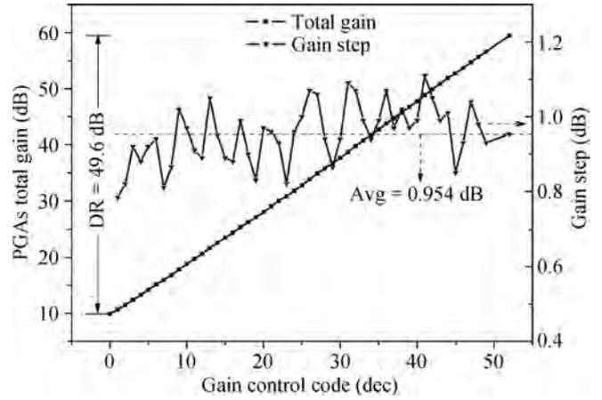
Fig. 12. The measured total gains and step of PGAs.
