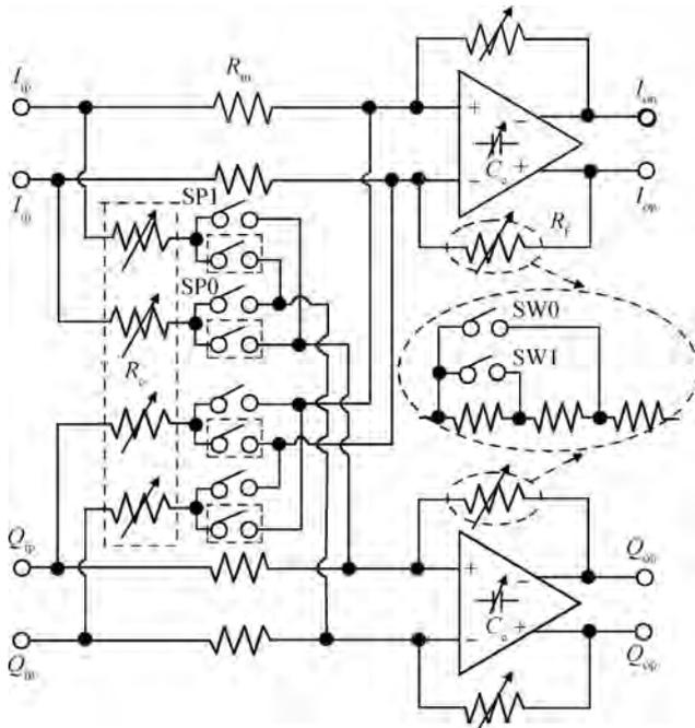
Fig. 5. The resistor feedback amplifier with I/Q phase calibration.
