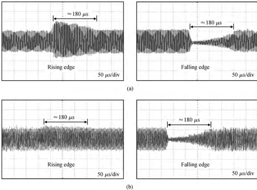
Fig. 13. PGA output signals with AM RF input with AGC at (a) 3.995 MHz and (b) 21.561 MHz.
