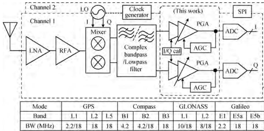
Fig. 1. The dual-channel multi-mode GNSS receiver incorporating I/Q AGC loops.
