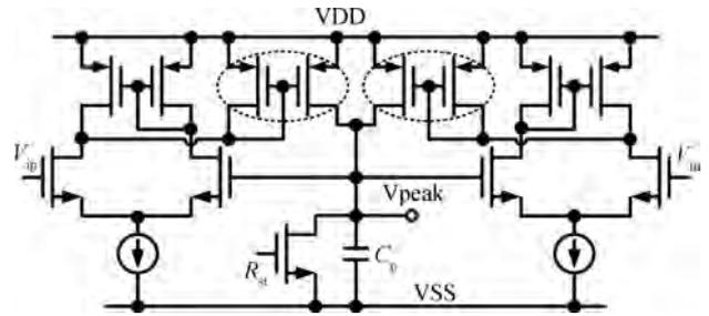
Fig. 7. The differential peak detector.
