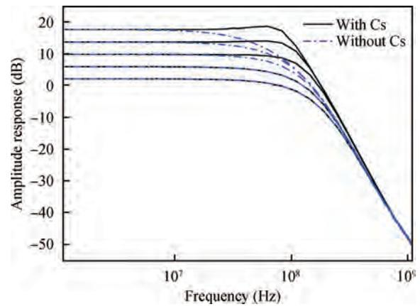
Fig. 4. The simulated amplitude response of the second stage (PGA2) with and without  $C_s$ .
