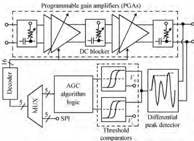
Fig. 2. Block diagram of the single AGC loop.
