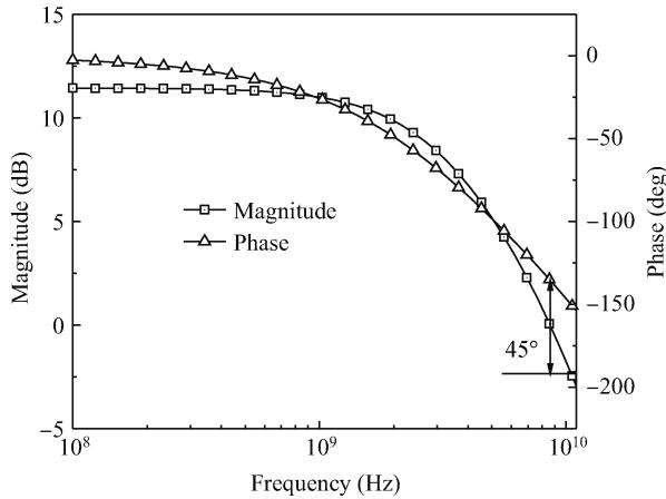
Fig. 8. The open loop frequency response of each fixed gain amplifier.
