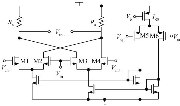
Fig. 2. The circuit of variable gain block.
