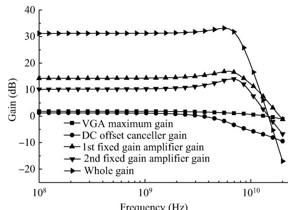
Fig. 7. The simulated frequency response of the amplifier gain.
