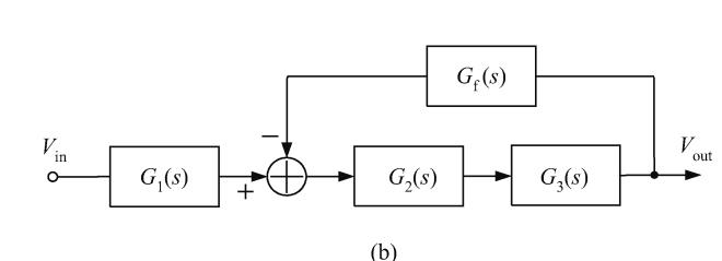
Fig. 6. (a) Circuit of the conventional third-order gain stages with active feedback. (b) The generic block diagram of the conventional structure.
