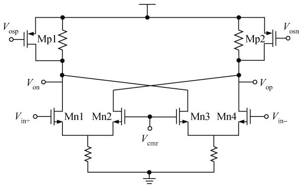
Fig. 5. Circuit of a DC-offset canceller.
