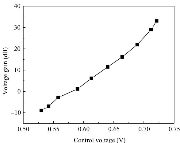
Fig. 10. Measured gain versus control voltage.
