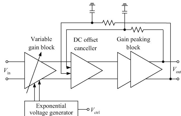
Fig. 1. Architecture of VGA.
