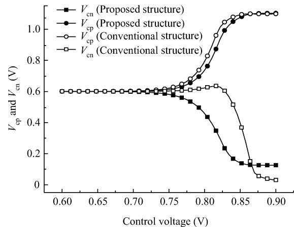
Fig. 4. Simulated results of  $V_{\text{cp}}$  and  $V_{\text{cn}}$  versus control voltage ( $V_{\text{ctrl}}$ ) in proposed and conventional structure respectively.
