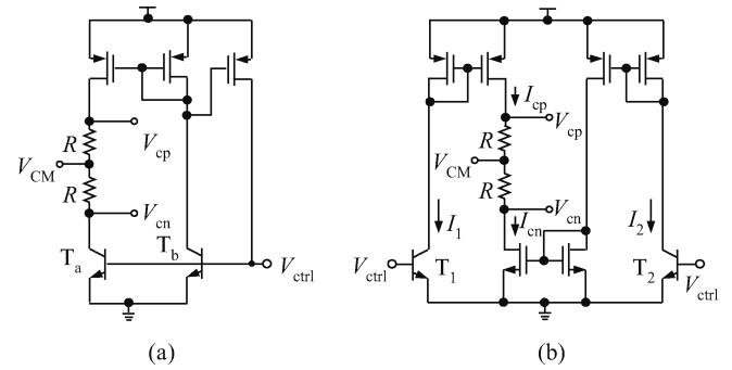
Fig. 3. Exponential voltage generator. (a) Conventional structure. (b) Proposed structure.
