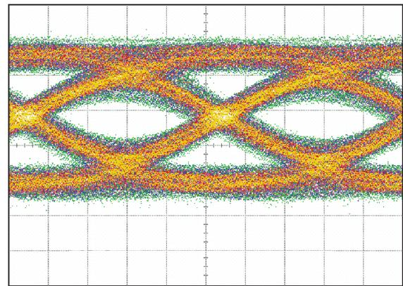
(b)  $V_{in} = 100$  mV<sub>pp</sub>Fig. 11. Measured  $10$  Gb/s  $2^{15}-1$  PRBS data single-ended output eye diagrams. H scale:  $20$  ps/div, V scale:  $66.3$  mV/div in (a),  $60.9$  mV/div in (b).
