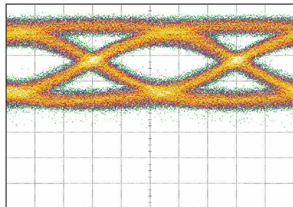
(a)  $V_{in} = 5$  mV<sub>pp</sub>
