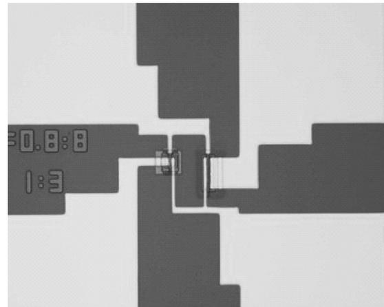
Fig. 4. Photograph of the strained CMOS inverter based on a  $\text{Si}_{1-x}\text{Ge}_x$  virtual substrate.
