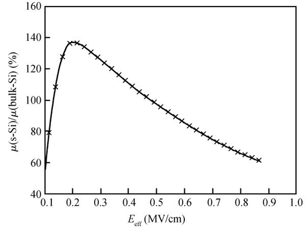
Fig. 7. Field-effect mobility ratio of the s-Si NMOSFET and the bulk-Si NMOSFET versus the effective field  $E_{\text{eff}}$  measured at  $V_d = 0.5 \text{ V}$ .
