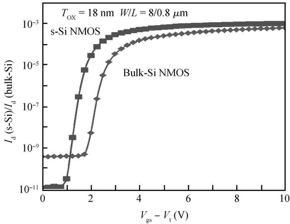
Fig. 5. Typical  $I_d$  versus  $V_{gs}-V_t$  characteristics for a  $0.8 \times 8 \mu\text{m}^2$  strained Si device and bulk-Si at  $V_{ds} = 0.5 \text{ V}$ .
