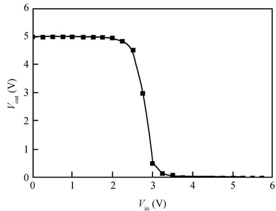
Fig. 8. Characteristics of the proposed inverter.
