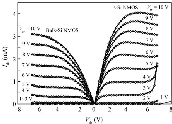
Fig. 6. Output characteristics of the strained NMOSFET and bulk Si NMOSFET at  $V_{gs} = 1-10 \text{ V}$ .
