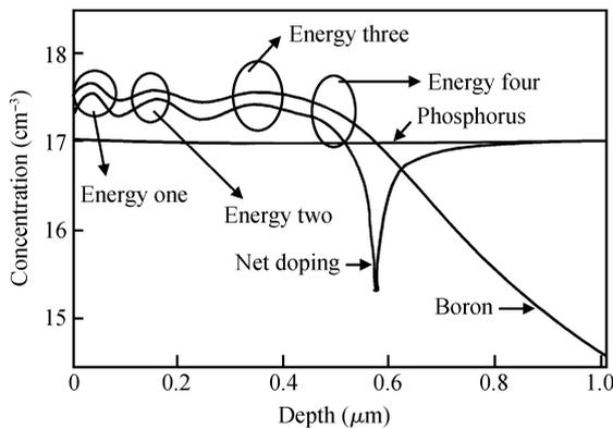
Fig. 3. Simulated distribution curves of the net doping and boron doping (boron is implanted with varied energy).
