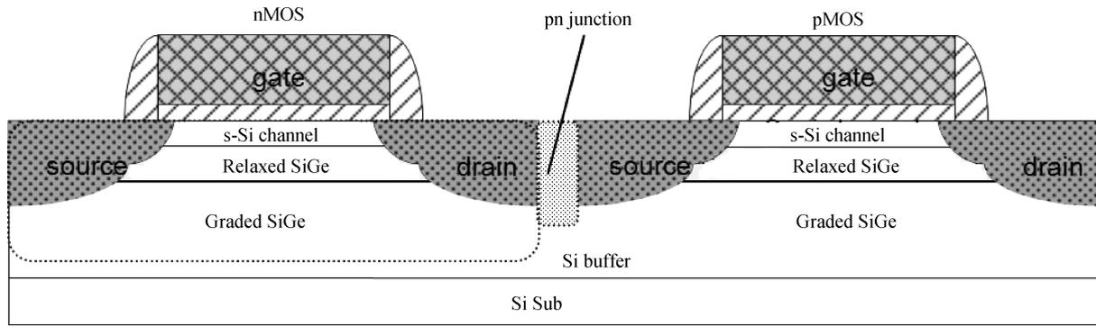
Fig. 1. Cross-section of the strained CMOS structure based on relaxed SiGe virtual substrate.
