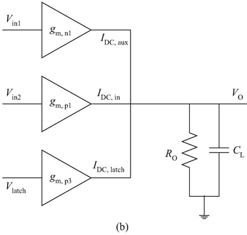
Fig. 1. (a) Circuit of the conventional delay cell. (b) The equivalent circuit of Fig. 1(a).
