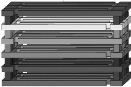
Fig. 4. Structure of the proposed MOM-capacitor.
