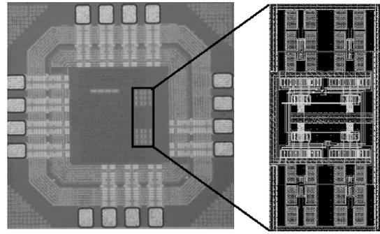
Fig. 5. Microphotograph of the fabricated ring VCO.
