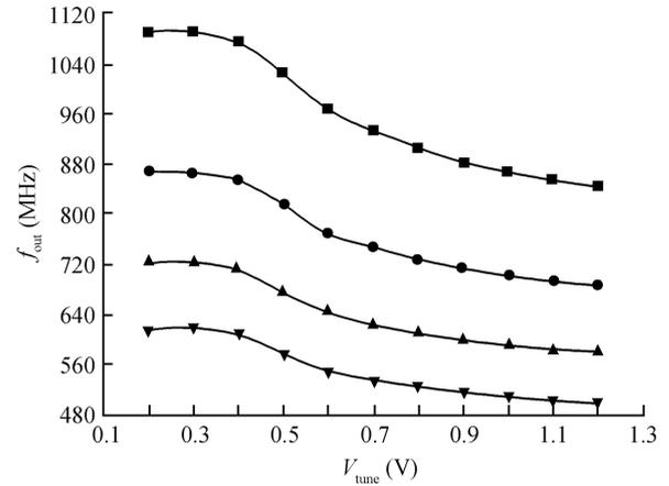
Fig. 6. The measured tuning curves of the proposed ring VCO.
