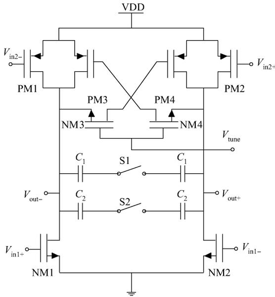
Fig. 3. Structure of the proposed delay cell.
