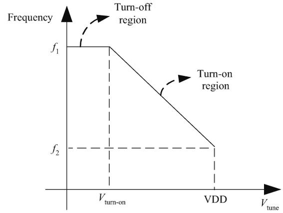
Fig. 2. Typical  $V-F$  curve of conventional ring VCO.
