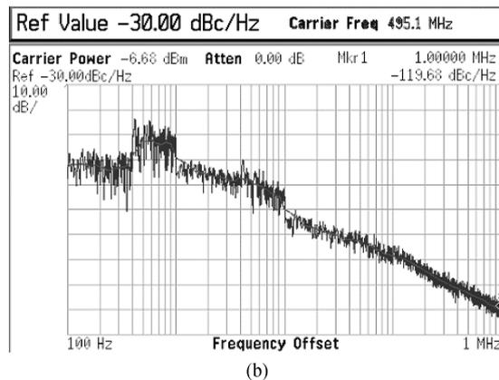
Fig. 7. The measured (a) output spectrum and (b) phase noise of the proposed ring VCO.
