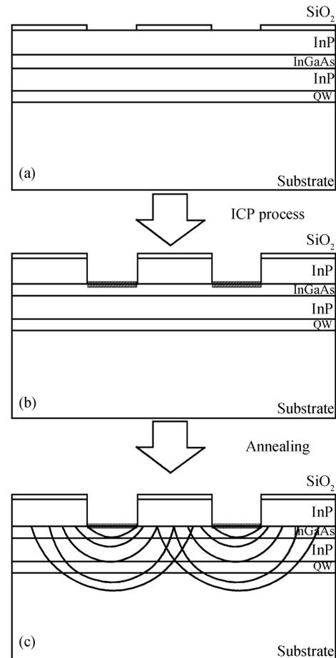
Fig. 3. A schematic diagram showing experimental process.
