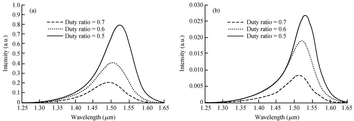
Fig. 4. (a) PL spectra of sample A with three different duty ratios before wet etching. (b) PL spectra of sample A after wet etching.
