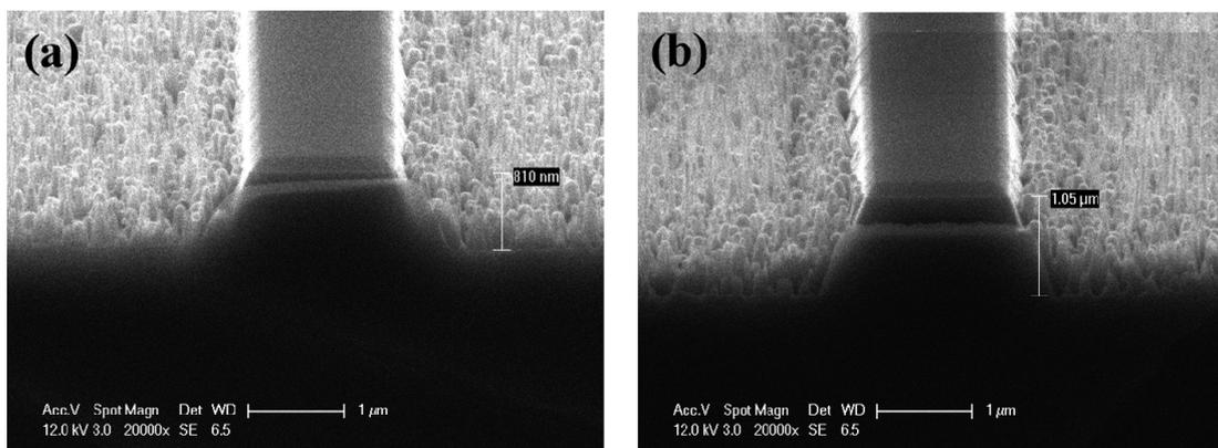
Fig. 6. The etching depth in the same sample with different duty ratios. (a) Duty = 0.7. (b) Duty = 0.8.
