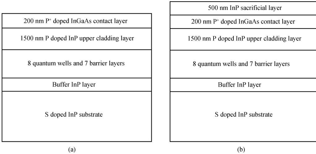
Fig. 1. Structure of (a) sample A and (b) sample B.
