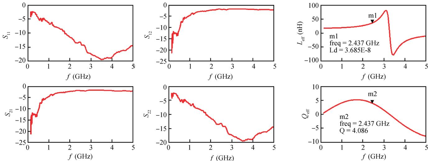
Fig. 8.  $S$ -parameters,  $L_{\text{eff}}$  and  $Q_{\text{eff}}$  test curve of the inductor.
