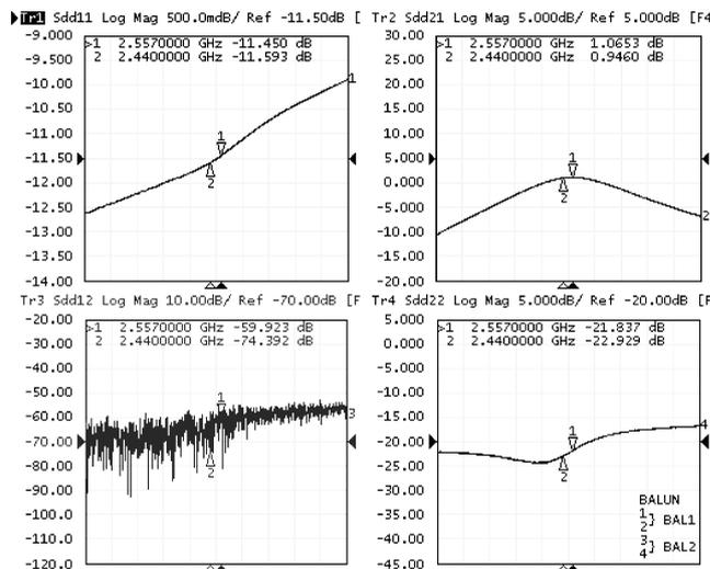
Fig. 11.  $S$ -parameter of the LNA at the low gain mode.
