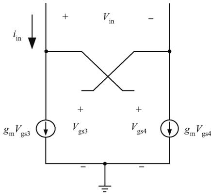
Fig. 5. Equivalent circuit of the second stage.
