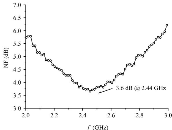
Fig. 12. Noise figure at high gain mode.
