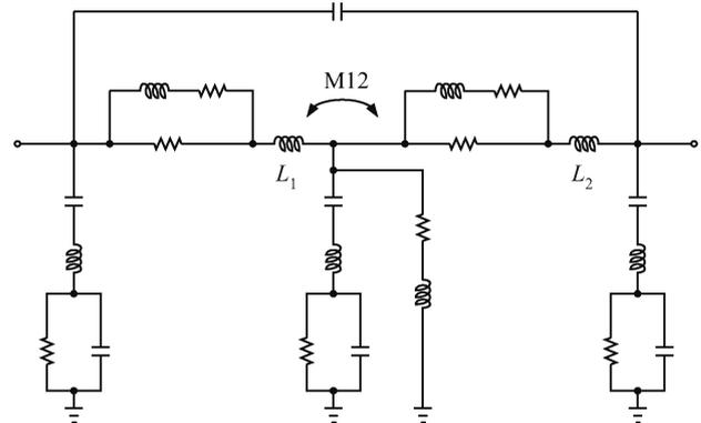
Fig. 4. The “double- $\pi$ ” circuit model for inductor  $L_d$ .
