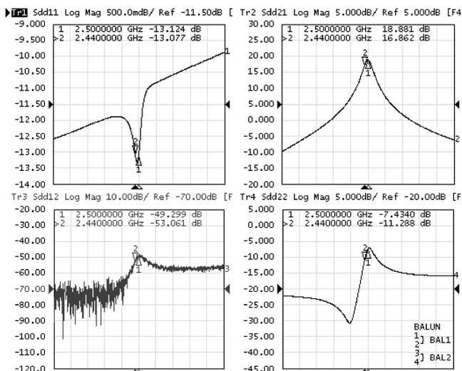
Fig. 10.  $S$ -parameter of the LNA at the high gain mode.
