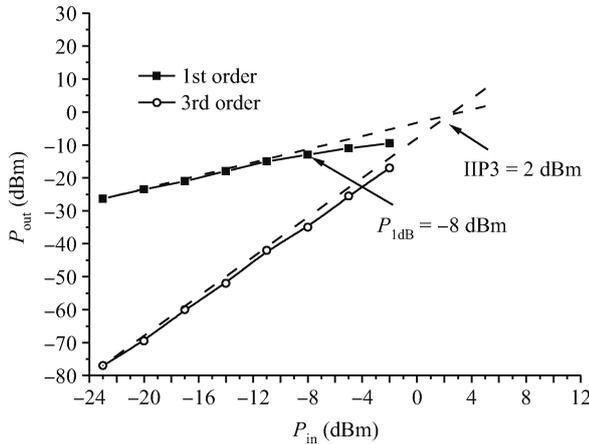
Fig. 8. IIP3 and  $P_{1dB}$  at low gain mode.
