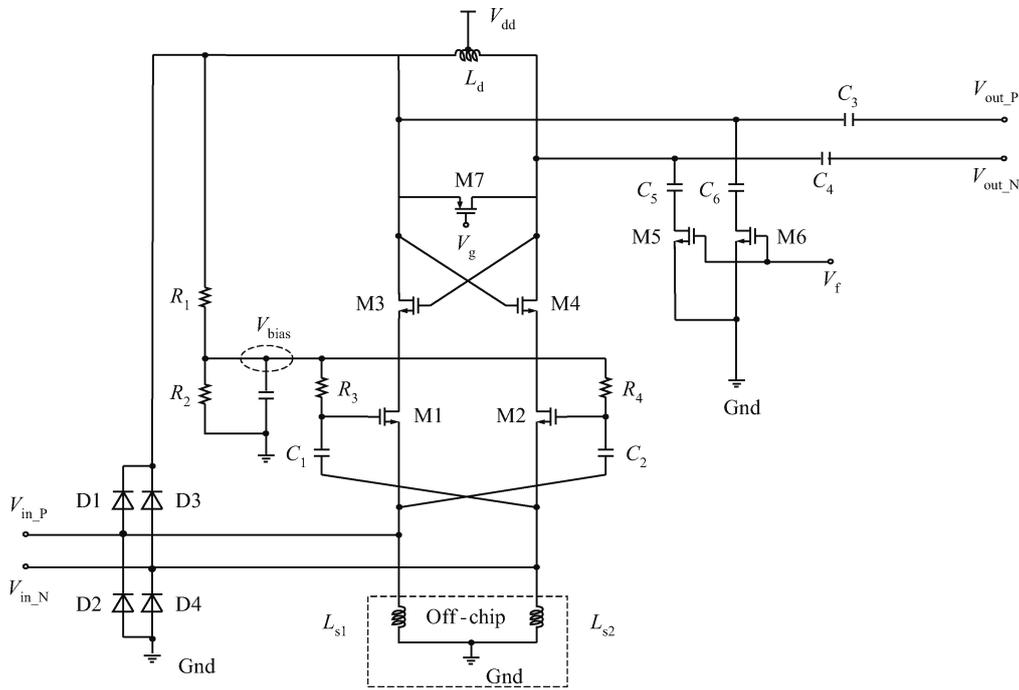
Fig. 1. Schematic of the LNA.
