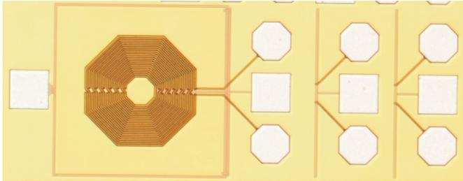
Fig. 7. Micro photo of the inductor for measurement.
