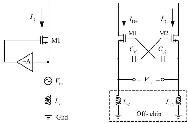
Fig. 6.  $G_m$ -boosted CG structure and capacitive cross-coupling CG LNA.
