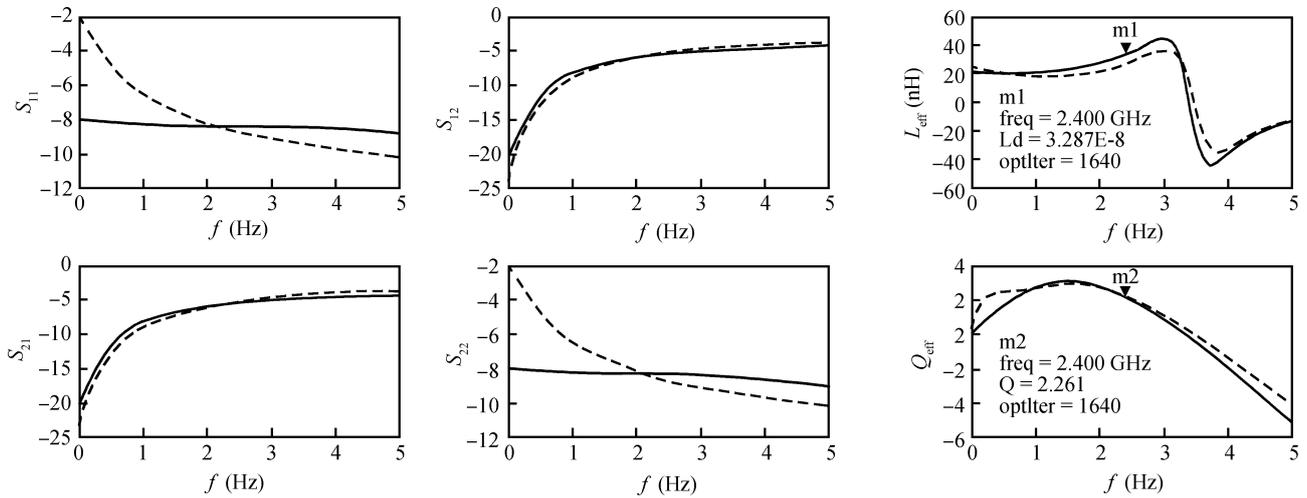
Fig. 3.  $S$ -parameters,  $L_{\text{eff}}$  and  $Q_{\text{eff}}$  simulation curve and iteration curve of the inductor model.
