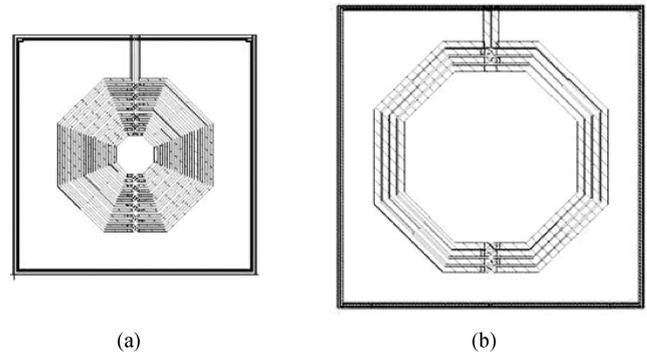
Fig. 2. (a) The inductor new designed compares with (b) the TSMC 0.18  $\mu\text{m}$  RF CMOS process provided largest inductor.
