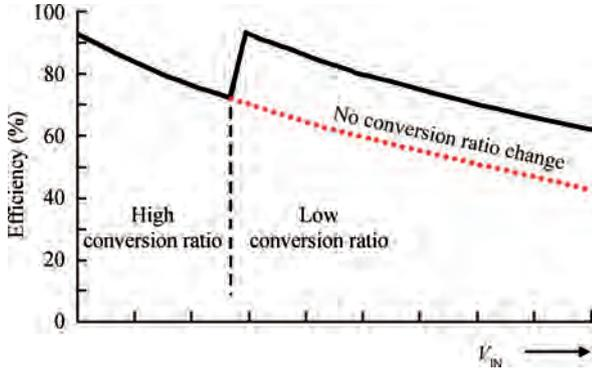
Fig. 2. Efficiency versus  $V_{in}$  for a fixed output voltage switched capacitor charge pump with different conversion ratios.
