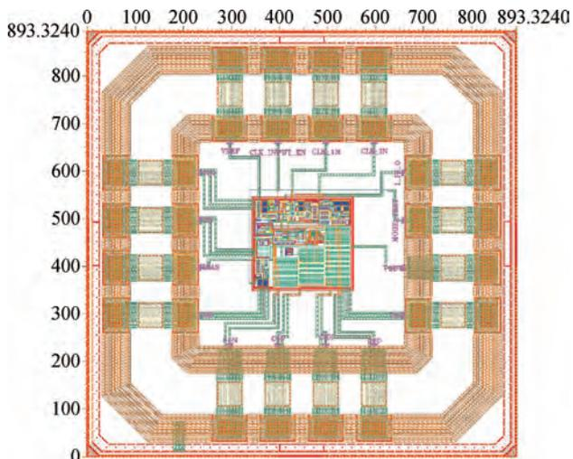
Fig. 9. Layout of the test chip in SMIC 40 nm CMOS process.
