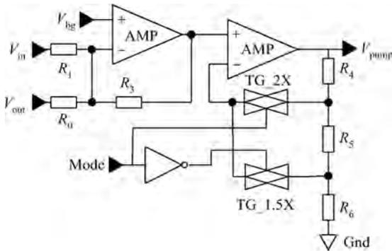
Fig. 4. Reference voltage  $V_{pump}$  generator.
