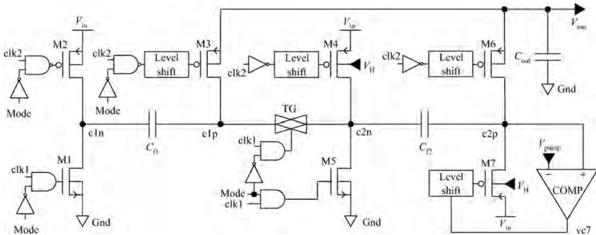
Fig. 3. The proposed charge pump is composed of  $V_0 - V_{DD}$  reference voltage generator, bulk bias selector, non-overlapping clock generator, hysteresis comparator and a conventional booster.
