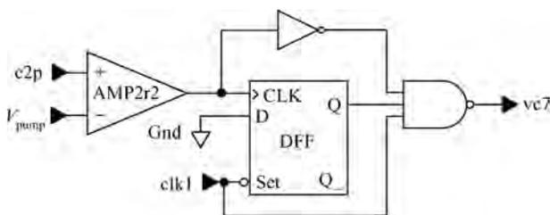
Fig. 7. Voltage comparator COMP.
