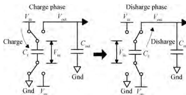
Fig. 1. The two operation steps of typical charge pump.
