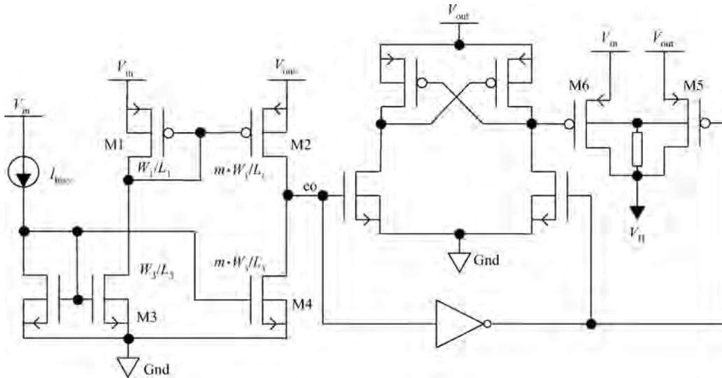
Fig. 5. Comparator circuit to bias bulk voltages at the higher of the input or output voltage.
