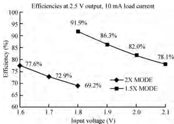
Fig. 11. Power efficiency at 10 mA load current versus  $V_{in}$ .
