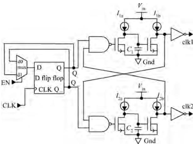
Fig. 6. Two phase non-overlapping clock generator.
