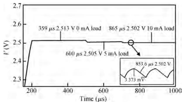
Fig. 10. Transient response of the charge pump with different load currents at a supply voltage of 1.8 V.
