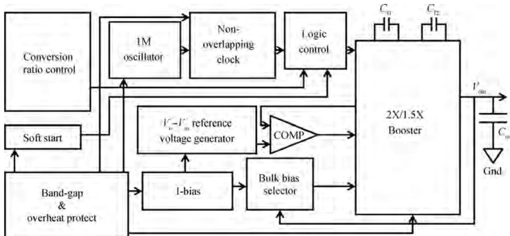
Fig. 8. The scheme of the charge pump.
