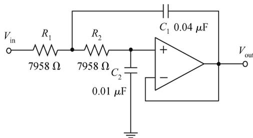
Fig. 4. Schematic of the Sallen and Key filter.
