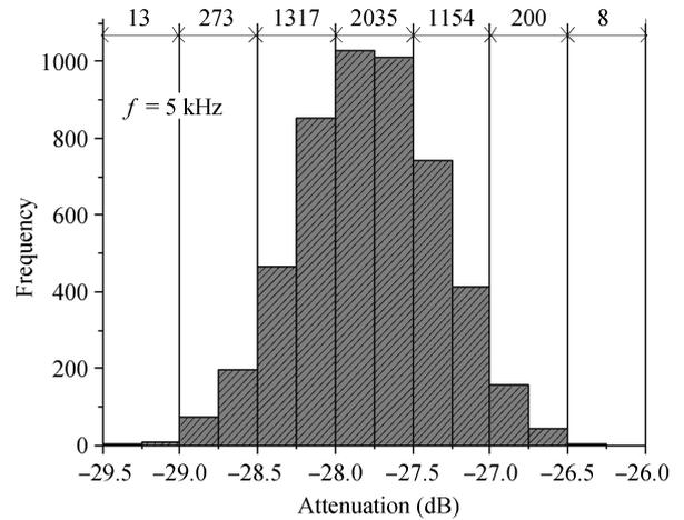
Fig. 5. Histogram of 5000 simulated performance data of the filter.
