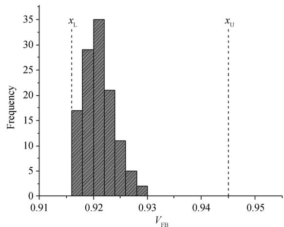
Fig. 6. Histogram of 120 voltage test data of qualified devices.
