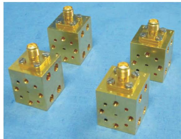
Fig. 5. Photo of the 150 GHz and 180 GHz SHM.
