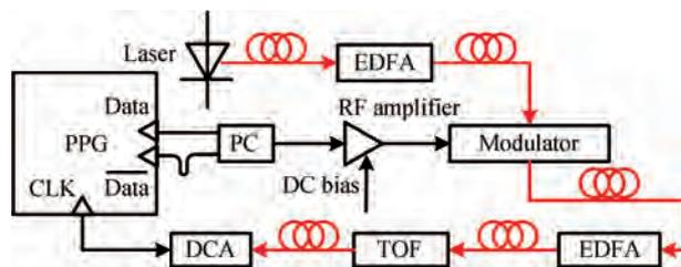
Fig. 3. Schematic of the experimental setup for the high-speed modulation experiment. PPG: pattern pulse generator; PC: power combiner; RF: radio-frequency; DCA: digital communication analyzer; EDFA: erbium-doped fiber amplifier; TOF: tunable optical filter; DC: direct current.
