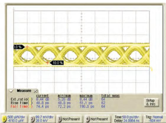
Fig. 5. Eye diagram of the optical modulator at the speed of 12.5 Gb/s.
