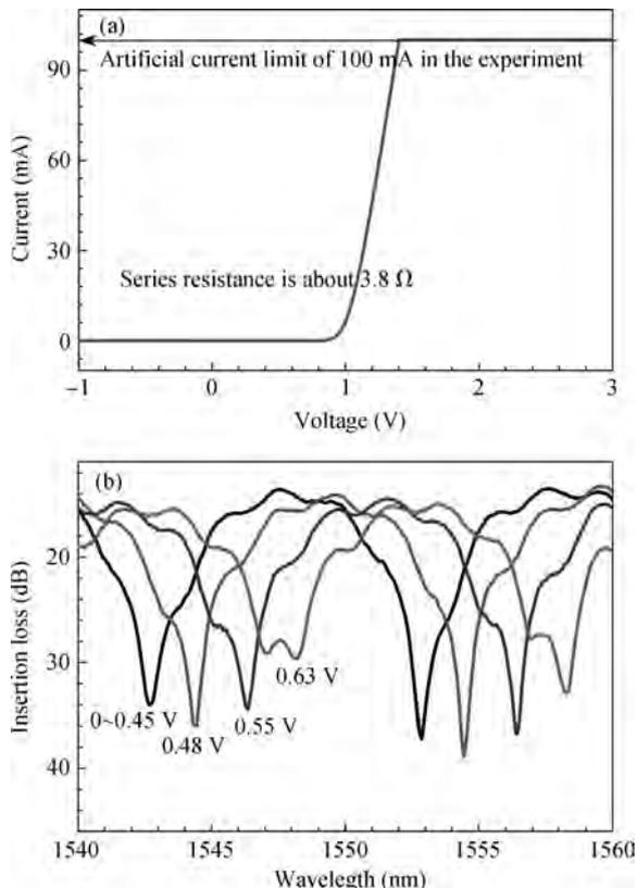
Fig. 2. (a) Current–voltage curve of the device. (b) Transmission spectra of the device with various voltages applied to the phase shifter.
