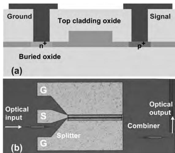
Fig. 1. (a) Cross-sectional view of a PIN junction waveguide phase shifter of the carrier-injection silicon Mach–Zehnder optical modulator. (b) Microscope image of the demonstrated silicon optical modulator.
