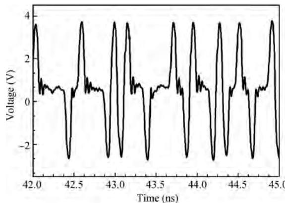
Fig. 4. Pre-emphasized electrical driving waveform of the device at 12.5 Gb/s.
