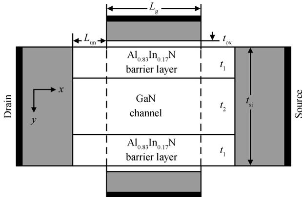
Fig. 1. Heterostructure underlap DG MOSFET showing underlap near the source and drain sides. The channel consists of an undoped narrow bandgap GaN ( $t_2 = 4$  nm) region and two wide bandgap  $\text{Al}_{0.83}\text{In}_{0.17}\text{N}$  ( $t_1 = 1$  nm) regions. Source/drain region doping is  $10^{20} \text{ cm}^{-3}$ , with 5 nm length. The gate length  $L_g = 18$  nm, the equivalent oxide thickness EOT is 1.2 nm, and body thickness  $t_{si} = 6$  nm.
