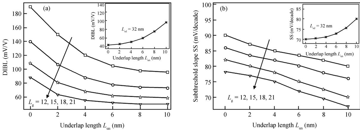
Fig. 5. (a) Variation of DIBL with  $L_{un}$ .  $L_g$  is varied from 12 to 21 nm in steps of 3 nm.  $L_{un}$  is varied from 0 to 10 nm in steps of 2 nm. (b) Dependence of SS on  $L_{un}$  for  $L_g = 12, 15, 18$  and 21 nm. Insets show the DIBL and SS variation with  $L_{un}$  for constant  $L_{sd} = 32$  nm.
