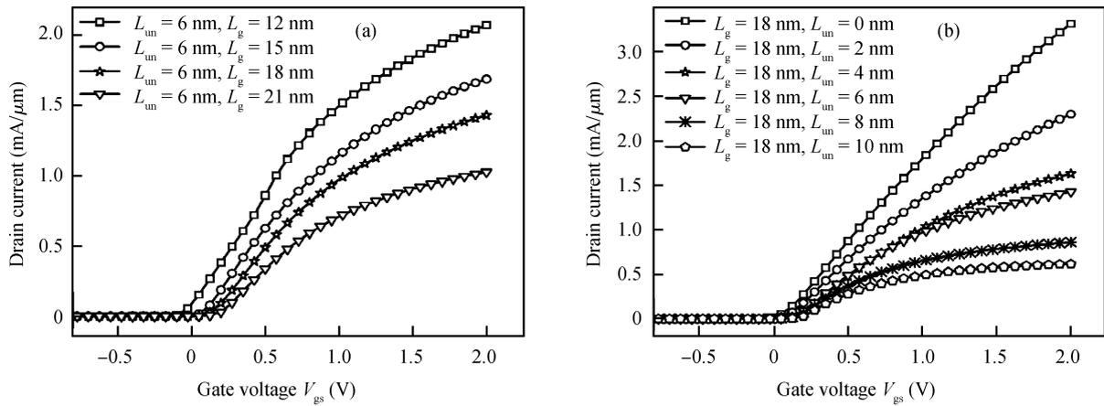
Fig. 4.  $I_D$  versus  $V_g$  characteristics for applied drain voltage is  $V_d = 1$  V for both devices. (a)  $L_g$  varied from 12 to 21 nm with  $L_{un} = 6$  nm. (b)  $L_{un}$  varied from 0 to 10 nm with constant  $L_g = 18$  nm.
