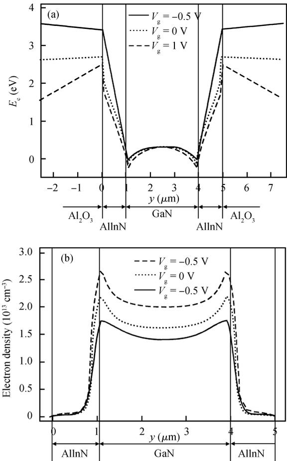
Fig. 2. (a) Simulated conduction band profile and (b) electron density distribution for  $V_{gs} = -0.5$  V, 0 V, 1 V, at the center of the gate along the direction normal to the transport direction for  $V_{ds} = 0$  V. 2DEG confined at the AlInN/GaN interface is observed.
