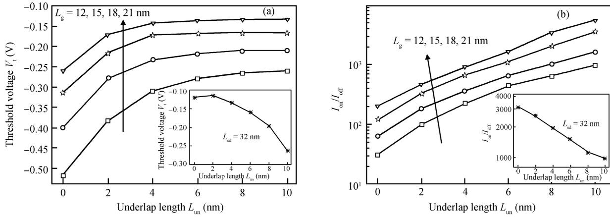
Fig. 6. (a) Variation of  $V_t$  with  $L_{un}$ .  $L_g$  is varied from 12 to 21 nm in steps of 3 nm.  $L_{un}$  is varied from 0 to 10 nm in steps of 2 nm. (b) Variation of  $I_{on}/I_{off}$  ratio on  $L_{un}$  for  $L_g = 12$  nm, 15 nm, 18 nm and 21 nm. Insets shows the  $V_t$  and  $I_{on}/I_{off}$  ratio variation with  $L_{un}$  for constant  $L_{sd} = 32$  nm.
