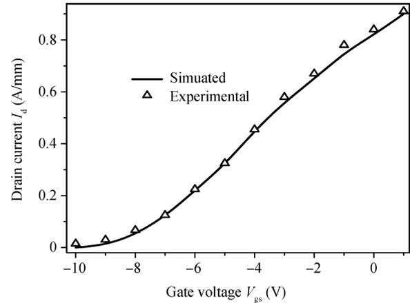
Fig. 3. Experimental (symbols) and simulated (solid lines) transfer characteristics for an AlInN/GaN buried channel MOSFET<sup>[13]</sup>, showing very good agreement between the two results.
