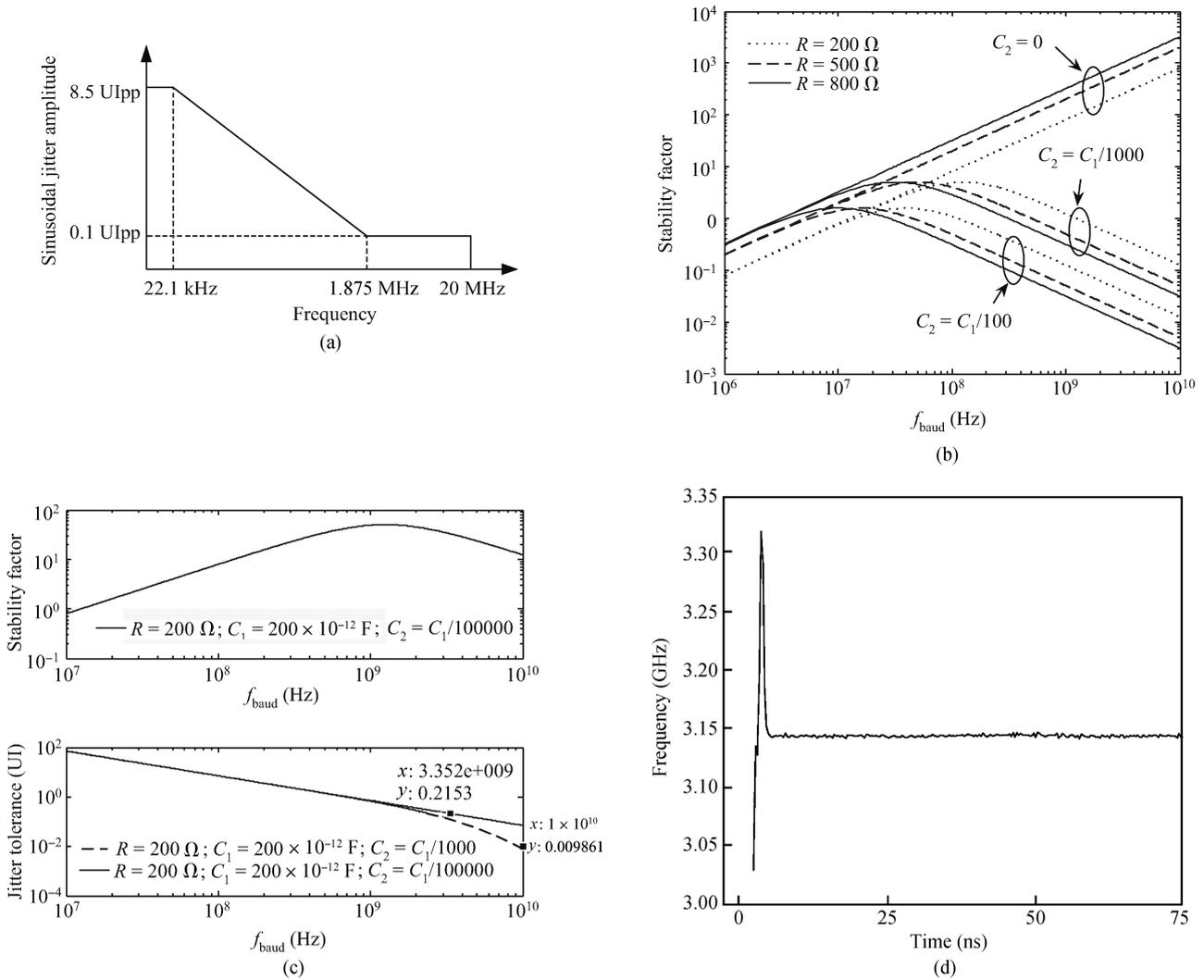
Fig. 6. The loop filter design. (a) Single tone sinusoidal jitter mask. (b) The stability factor versus  $R$  and  $C_2$ . (c) The jitter tolerance versus  $C_2$ . (d) The convergence curve of the frequency.
