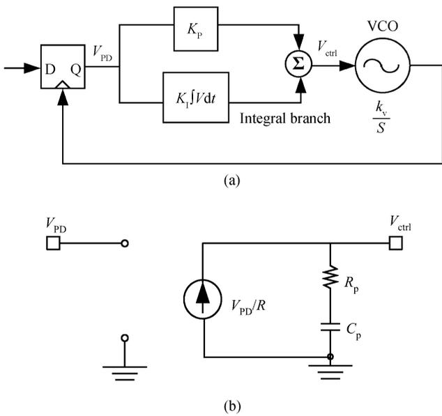
Fig. 2. (a) The two-order bang-bang PLL. (b) The nonlinear equivalent model.
