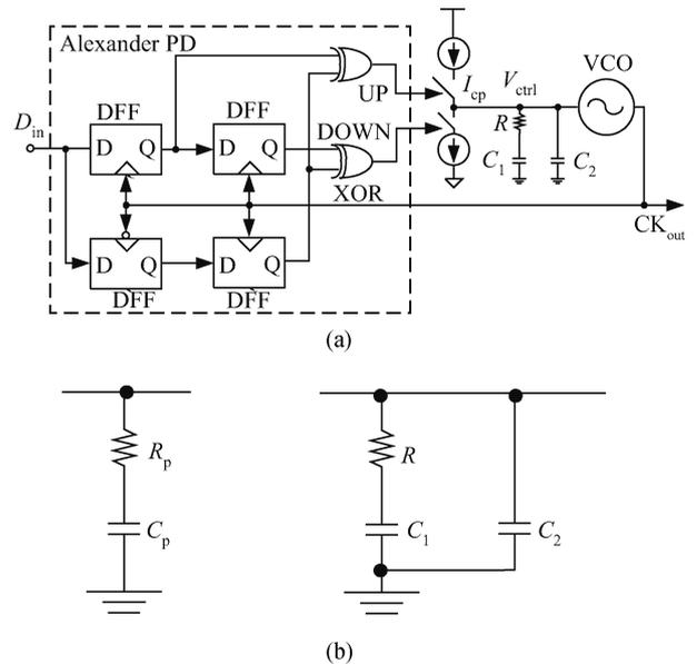
Fig. 3. (a) The third-order bang-bang PLL diagram. (b) The equivalence between the 1st-order filter and the 2nd-order filter.
