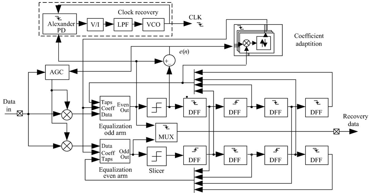
Fig. 1. The SerDes core with a clock recovery.
