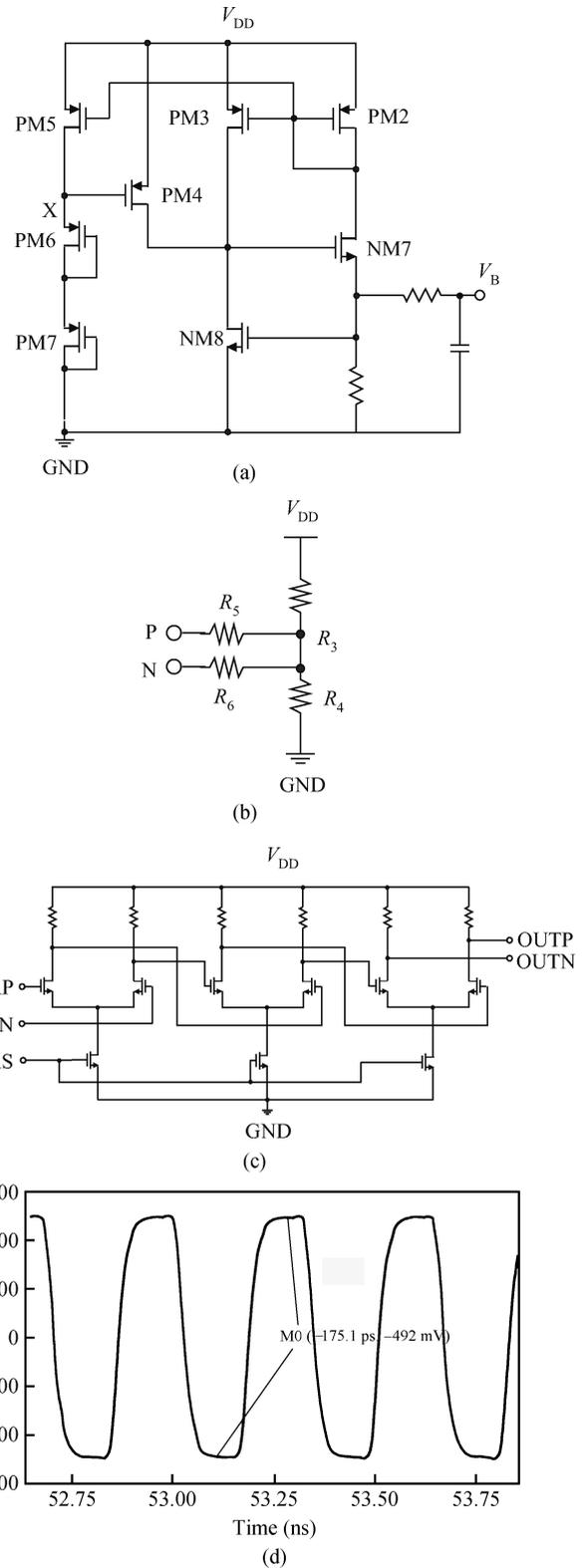
Fig. 7. Circuit diagram of the current resource and buffer. (a) The schematic of the current source. (b) The input buffer and impedance-matching circuit. (c) The schematic of the data-out buffer. (d) Output amplitude.
