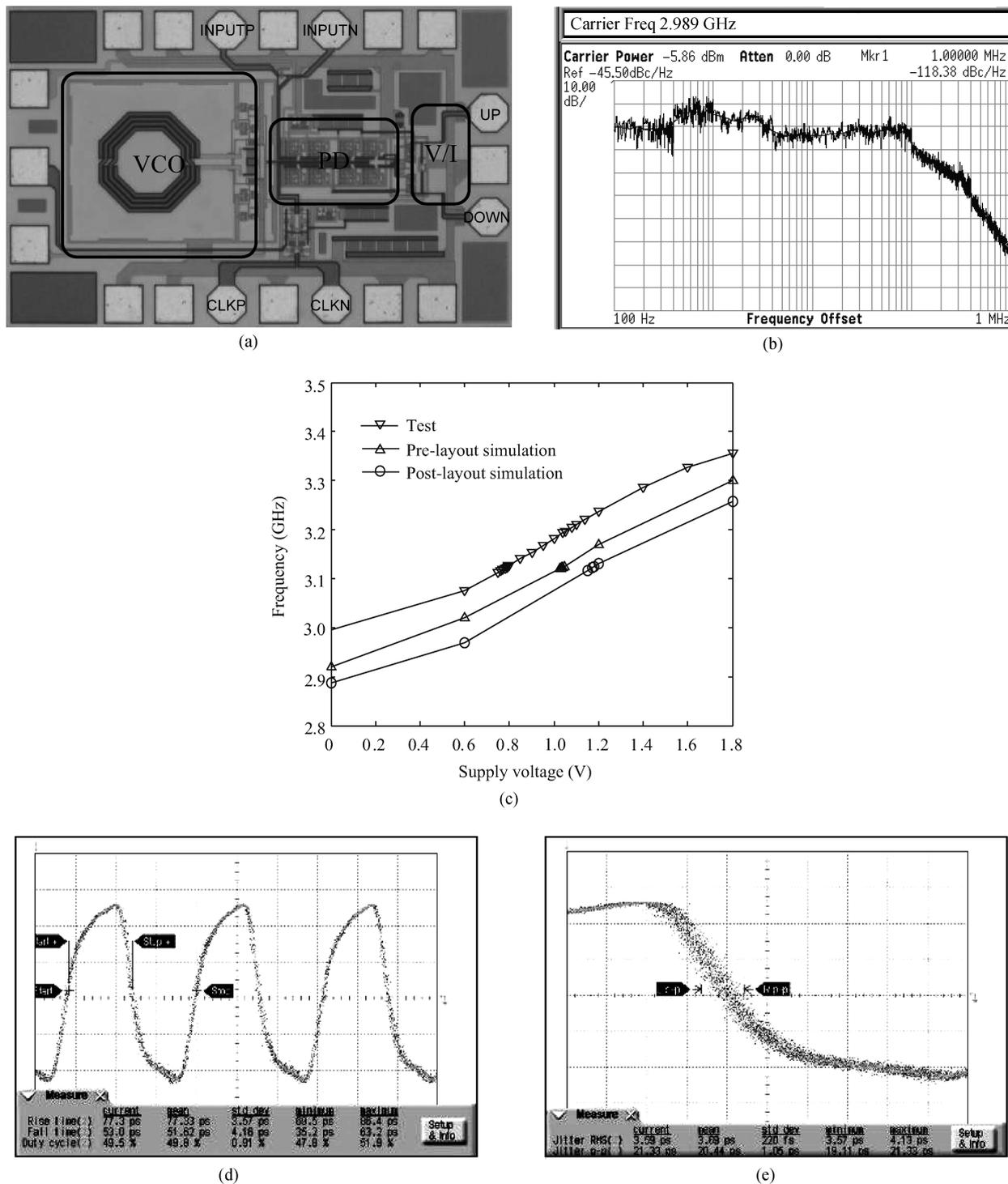
Fig. 8. The test results. (a) The chip photomicrograph. (b) The phase noise curve. (c) The VCO frequency voltage control curves. (d) The clock signal recovered. (e) the jitter in the falling edge.
