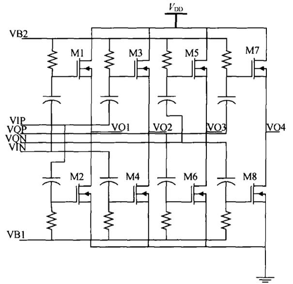
Fig. 4 Core schematic of phase and amplitude calibration circuit
