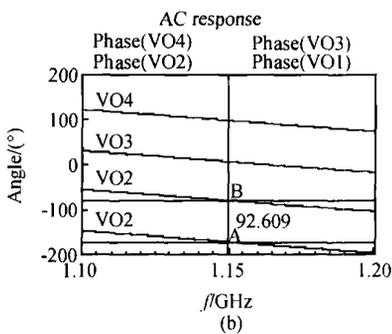
Fig. 8 Simulated phase error without (a) and with PMCC (b) with by Spectra RF
