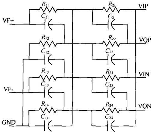
Fig. 3 Schematic of second-order poly phase network
