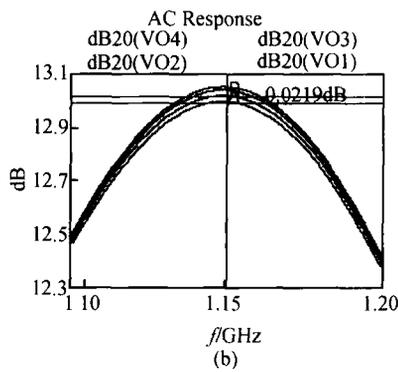
Fig. 7 Simulated amplitude difference without (a) and with PMCC (b) by Spectra RF
