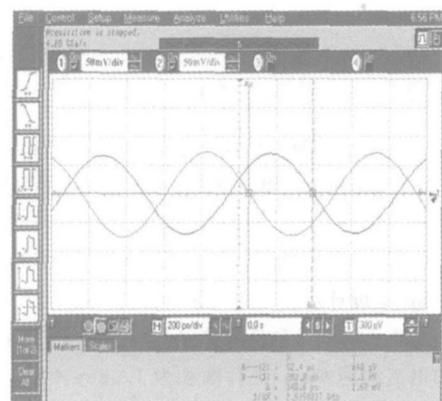
Fig. 11 Measured output signals in two adjacent branches
