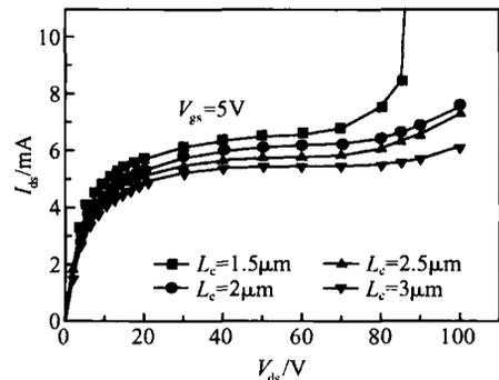
Fig. 5 Output characteristics of different channel
