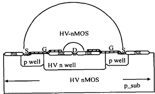
Fig. 8 Self-enclosed HV-nMOS
