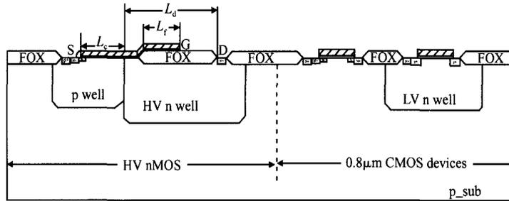
Fig. 1 Schematic cross section of high-voltage nMOS device
