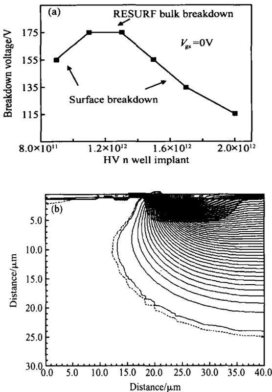
Fig.2 MEDICI simulation results (a) Breakdown voltage versus HV n well doping; (b) Equipotential contours of HV-nMOS ( $V_{gs} = 0V, V_{ds} = 170V$ )
