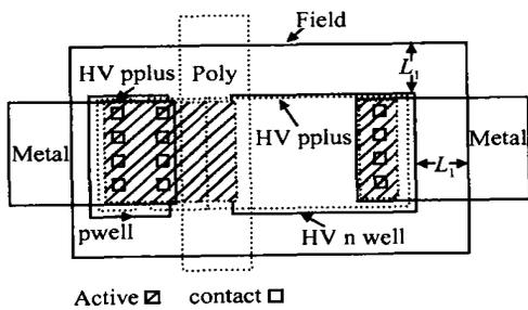
Fig. 6 Layout of HV-nMOS
