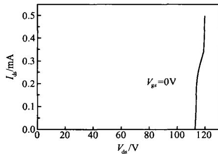
Fig. 4 Breakdown voltage of HV-nMOS devices
