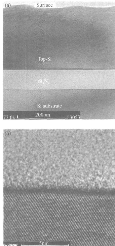
Fig.1 XTEM image (a) and HRTEM image (b) of the new SOI structures
