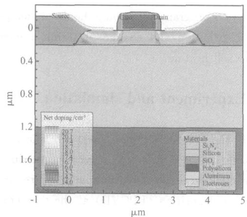
Fig. 3 Structure distribution of the MOSFET device
