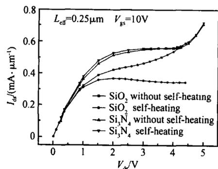
Fig. 4 Simulated output characteristics of SOI and SOSN devices
