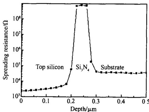
Fig. 2 Spreading resistance profile of the SOI structures
