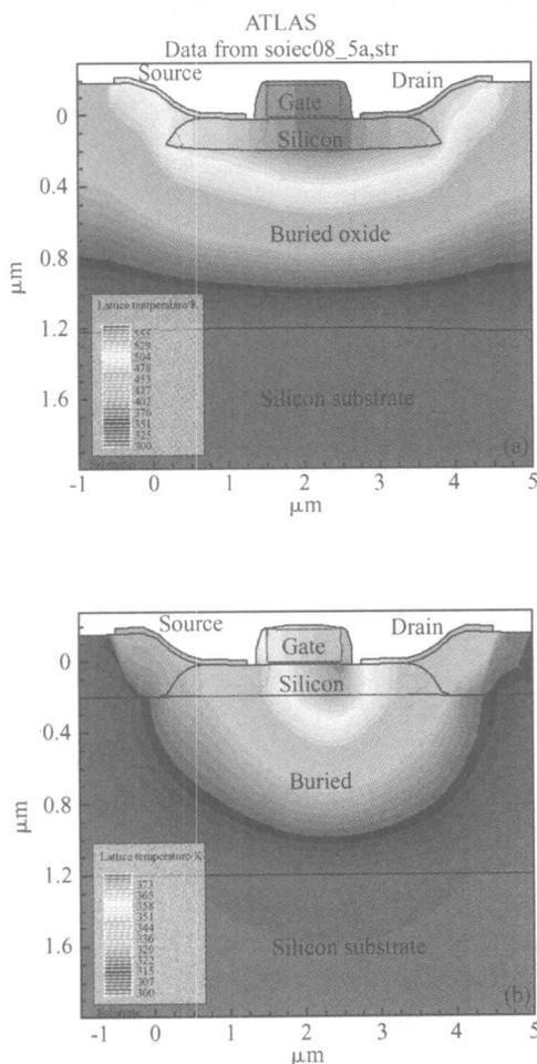
Fig. 5 Simulated temperature distributions of SOI (a) and SOSN (b) devices
