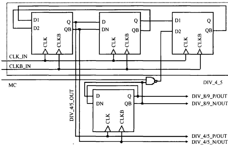
Fig. 2 Block diagram of the high speed dual-modulus prescaler
