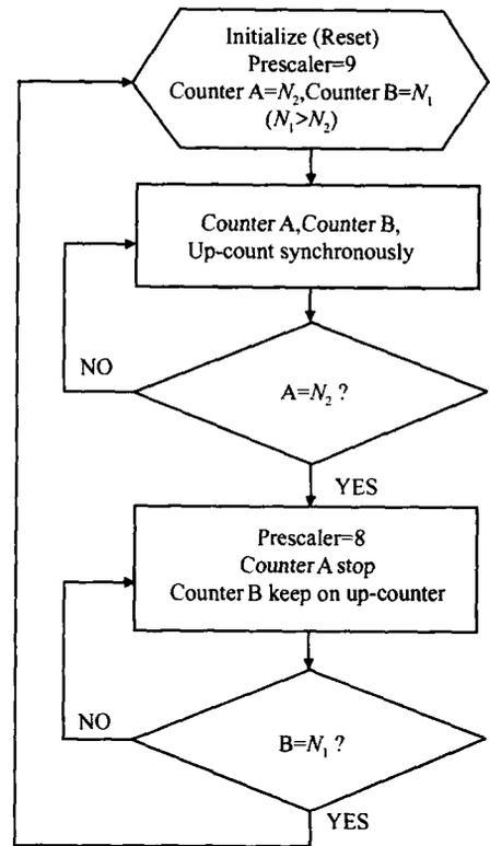
Fig. 5 Behavior flow diagram of down scalers
