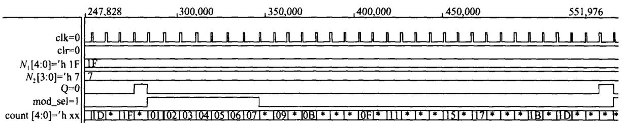
Fig. 6 Post-simulation waveforms of 9-bits programmable divider
