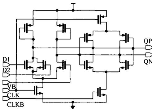
Fig. 3 D-latch architecture with 'OR' logic input
