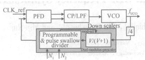
Fig. 1 Block diagram of the PLL-type frequency synthesizer
