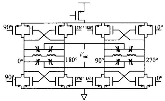
Fig. 1 Circuit diagram of QVCO
