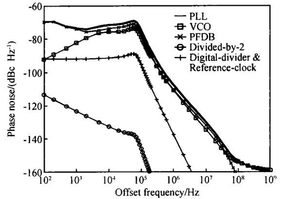
Fig. 5 Simulation results of the synthesizer's phase noise with a linear phase domain model
