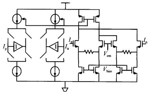
Fig. 2 Circuit diagram of differential charge pump
