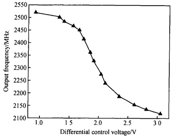
Fig. 7 Tuning characteristic of the VCO when DC-CA is biased at its maximum value
