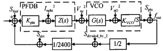
Fig. 4 Linear phase domain model for the frequency synthesizer simulation
