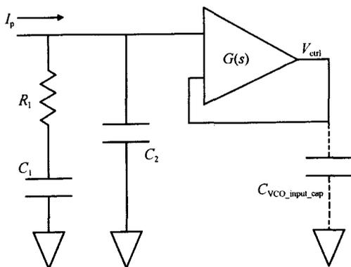
Fig. 3 Topology of a equivalent third order loop filter
