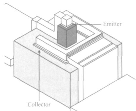
Fig. 1 Schematic mesa structure of the DBRTD
