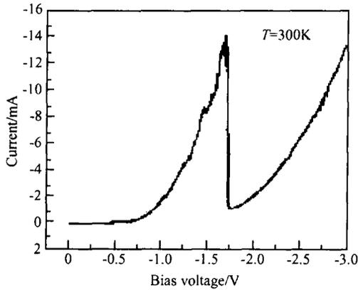
Fig. 2 *I-V* curve of RTD with a  $4\mu\text{m} \times 4\mu\text{m}$  emitter PVCr = 13.98 with  $I_p = -0.014309\text{A}$ ,  $V_p = -1.68\text{V}$ ,  $I_v = -0.0010236\text{A}$ ,  $V_v = -1.707\text{V}$
