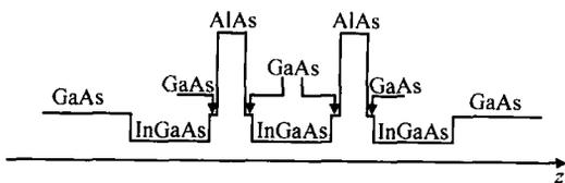
Fig. 3 Schematic conduction band diagram with *z* direction that parallels the current one in DBRTD
