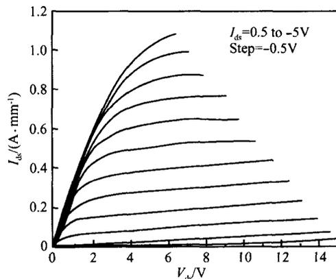
Fig. 5  $I_{ds}$ - $V_{ds}$  characteristics of a typical AlGaIn/GaN HEMT grown on sapphire substrate with gate length and width of 0.2  $\mu\text{m}$  and 0.8mm, respectively
