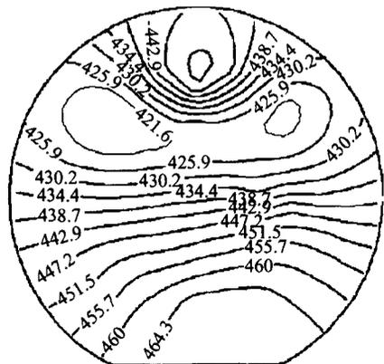
Fig. 4 Sheet resistance mapping of the grown 50mm AlGaIn/GaN HEMT wafer
