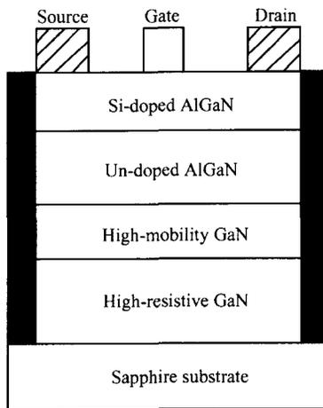
Fig. 1 Schematic cross section of an AlGaIn/GaN HEMT
