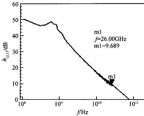
Fig. 7 Small signal RF characteristic of the  $0.2\mu\text{m} \times 40\mu\text{m}$  AlGaIn/ GaN HEMT device
