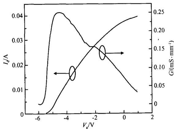
Fig. 6 DC transfer characteristics of a typical AlGaIn/GaN HEMT grown on sapphire substrate with gate length and width of 0.2 and 40  $\mu\text{m}$ , respectively
