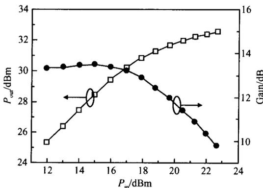
Fig. 8 Power performance of the  $0.2\mu\text{m} \times 0.8\text{mm}$  AlGaIn/ GaN HEMT at 8GHz. The device was biased at  $V_{ds} = 30\text{V}$ .
