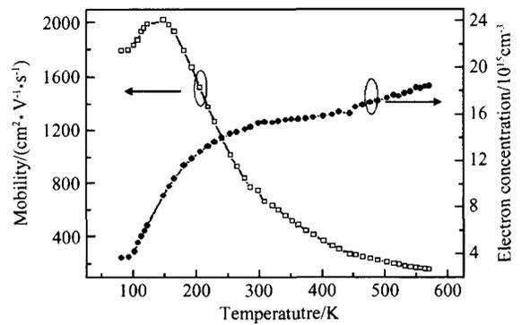
Fig. 2 Electron mobility and concentration as a function of sample temperature for an unintentionally doped 2.5mm thick bulk GaN epilayer on sapphire
