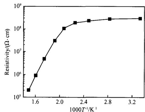
Fig. 3 Temperature dependence of the electrical resistivity of the 2.8 $\mu\text{m}$  thick GaN buffer layer grown on sapphire substrates by MOCVD
