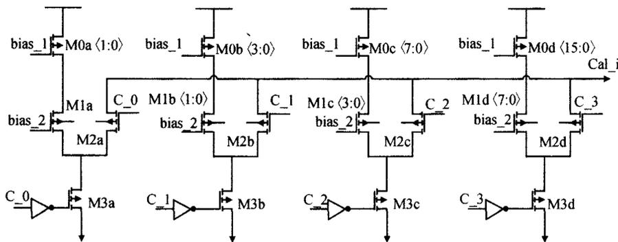
Fig. 5 Core structure of DAC\_2
