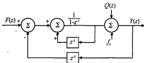
Fig. 8 First-order sigma-delta modulator
