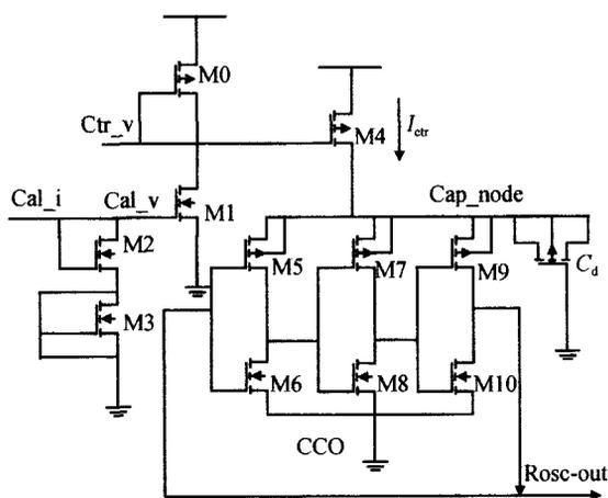
Fig. 6 Core structure of VCO
