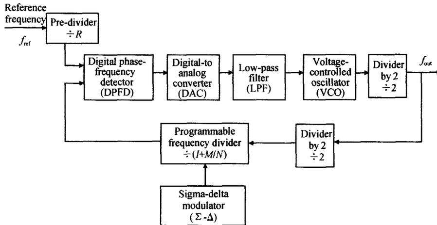
Fig. 1 DPLL functional block diagram
