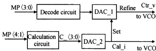
Fig. 4 Block diagram of self-calibration
