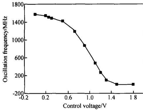
Fig. 7 VCO frequency versus the control voltage Ctr\_v
