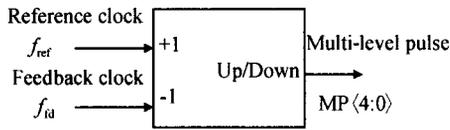
Fig. 2 Digital frequency-phase detector
