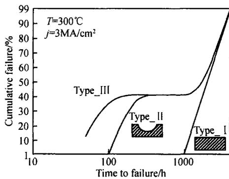
Fig. 5 Simulated time to cumulative failure distributions of different element types Inserts :diagrams of different types of elements
