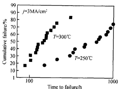
Fig. 3 Time to cumulative failure distributions of samples with pre-existing surface-defects (Set \_ B) under different temperature stress The activation energy is around 0. 74 ±0. 02eV.
