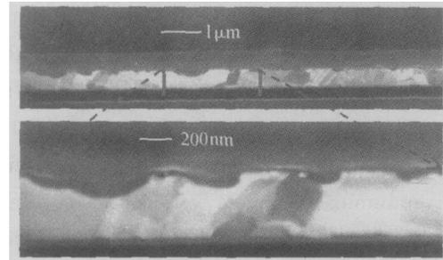
Fig. 4 Postmortem FIB analysis of samples with pre-existing surface-defects (Set \_ B)
