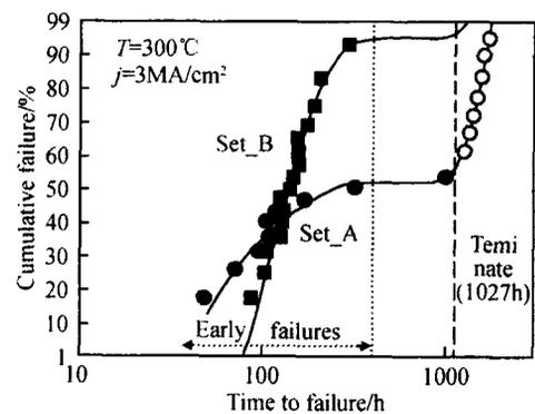
Fig. 2 Time to cumulative failure distributions of samples without (Set \_ A) and with (Set \_ B) pre-existing surface-defects Symbols are experiment results ,and curves are simulated. Empty circles are surviving samples after 1027h.
