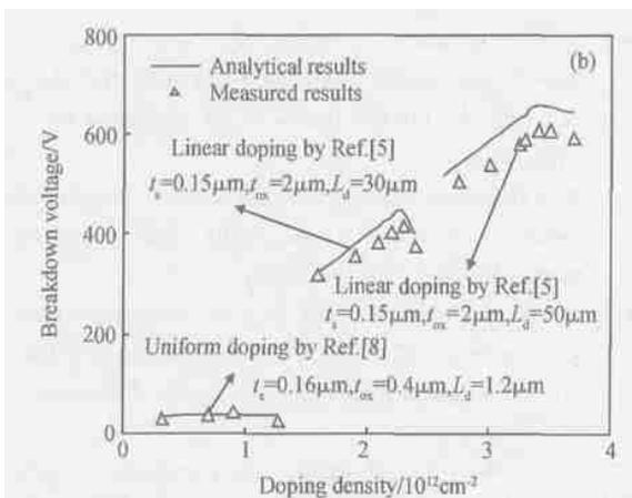
Fig. 4 Numerical ,experimental ,and analytical results of the breakdown as a function of the concentration slope (a) and the drift charge density (b)
