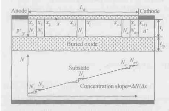
Fig. 1 Schematic cross section of SOI RESURF device with step doping profile in the drift region
