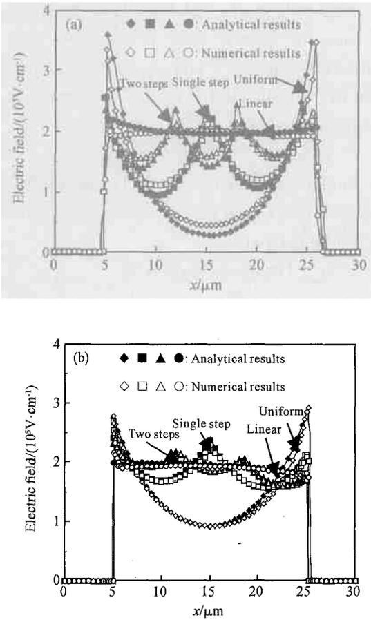
Fig. 2 Profiles of optimal surface electric field near breakdown for the different steps number (a)  $t_s = 1\mu\text{m}$ ,  $t_{ox} = 3\mu\text{m}$ ; (b)  $t_s = 3\mu\text{m}$ ,  $t_{ox} = 3\mu\text{m}$
