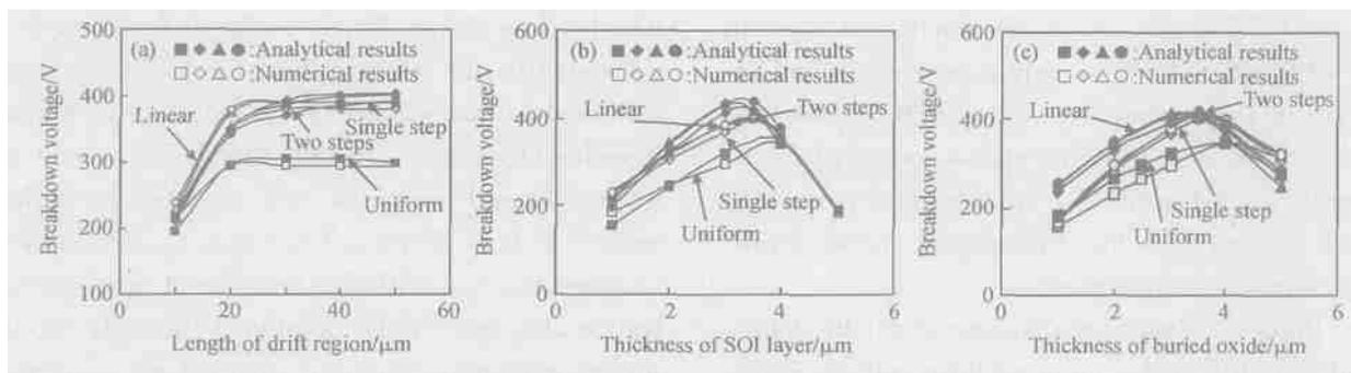
Fig. 5 Breakdown voltage as a function of drift region length (a), thickness of SOI layer (b), and thickness of buried oxide layer (c)
