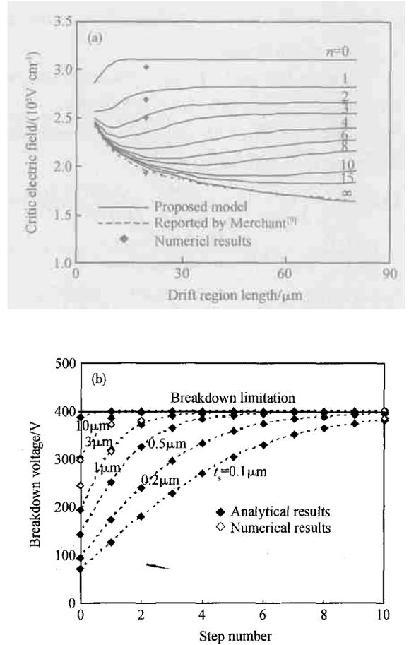
Fig. 3 Critic electric field and breakdown voltage for different steps numbers (a) Critic electric field as a function of drift region length; (b) Breakdown voltage as a function of steps number
