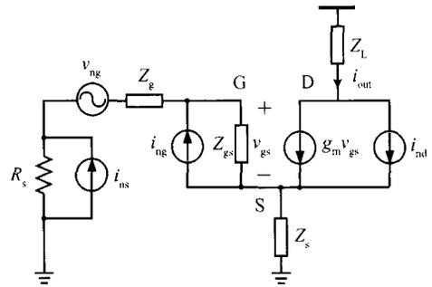
Fig. 2 Generic small-signal model for LNA noise analysis
