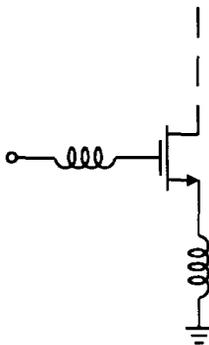
Fig. 1 Source inductive degeneration LNA architecture
