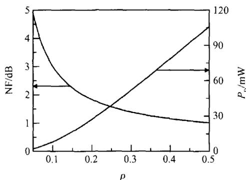
Fig. 3 Optimum NF for fixed  $G_m$  optimization and corresponding  $P_D$  versus  $\rho$
