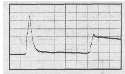
Fig. 4 Waveform of complex mode X: 50ns/div, Y: 500mV/div
