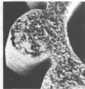
Fig. 3 Close-up of the microgear with rough surface
