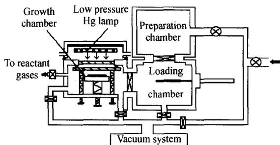
Fig. 1 Schematic of UV/UHV/CVD system
