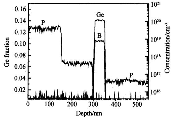
Fig. 3 SIMS profile of n-Si/i-Si<sub>0.86</sub>Ge<sub>0.14</sub>/p<sup>+</sup>-Si<sub>0.86</sub>Ge<sub>0.14</sub>/i-Si<sub>0.86</sub>Ge<sub>0.14</sub>/n-Si
