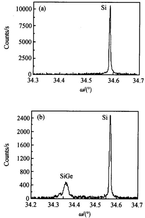
Fig. 2 X-ray diffraction of SiGe grown at 300 °C (a) and 450 °C (b)
