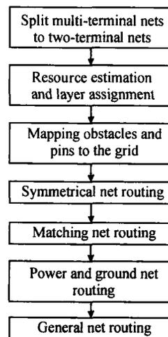
Fig. 7 Algorithm flow of RT sub-system
