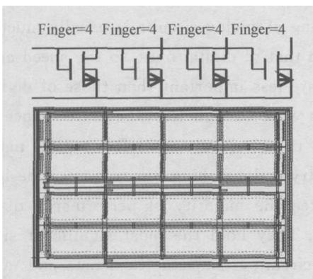
Fig. 5 Schematics of current mirror and 2D common centroid layout
