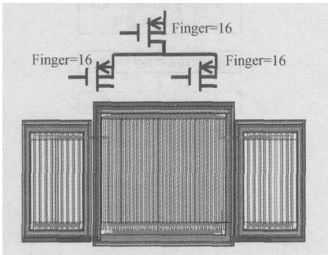
Fig. 4 Schematics of differential pairs and 1D common centroid layout
