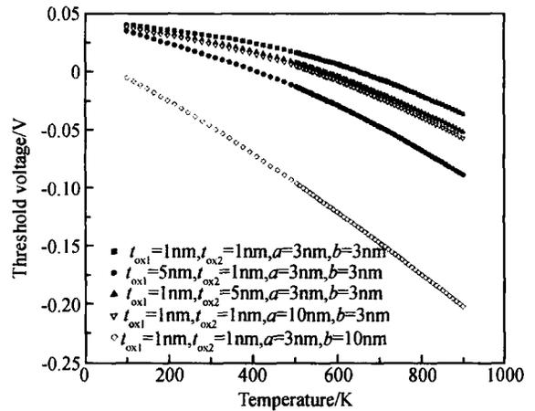
Fig. 4 Threshold voltage  $V_T$  versus temperature  $T$  with different  $t_{ox1}$ ,  $t_{ox2}$ ,  $a$ , and  $b$   $t_{ox3} = 30nm$ .
