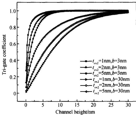
Fig. 3 Tri-gate coefficient  $H$  versus channel height  $a$  with different  $t_{ox2}$  and  $b$   $t_{ox1} = 1nm$  and  $t_{ox3} = 30nm$ .
