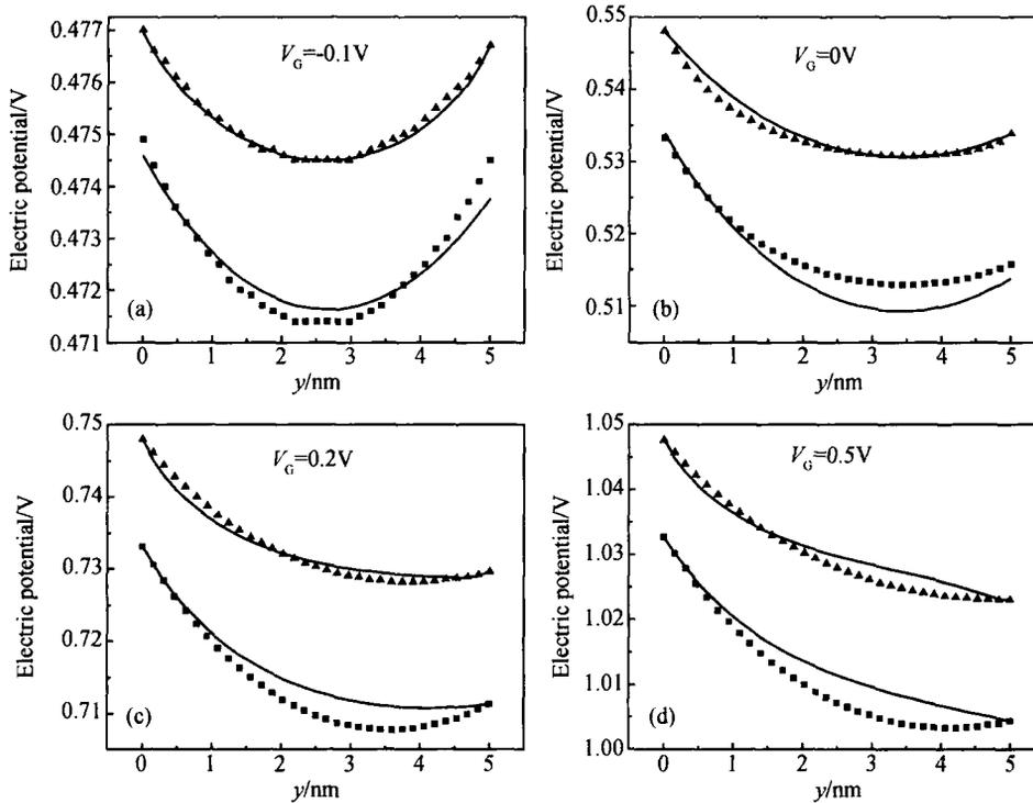
Fig.2  $\phi(-b/2, y)$  and  $\phi(0, y)$  profiles along height direction at various gate voltages  $a = b = 5nm, t_{ox1} = t_{ox2} = 1nm$  and  $t_{ox3} = 25nm$ . Symbols stand for numerical simulation results (triangles for  $\phi(-b/2, y)$  and squares for  $\phi(0, y)$ ) while solid lines stand for analytical results.
