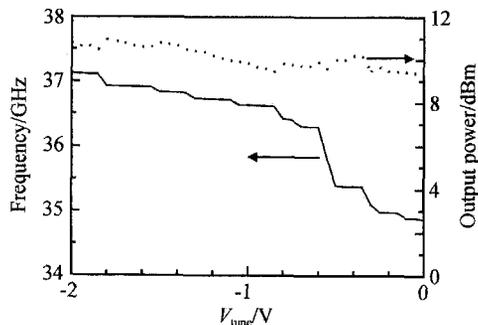
Fig. 4 Oscillating frequency and output power tuning curves
