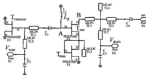
Fig. 2 Schematic of the designed MMIC VCO
