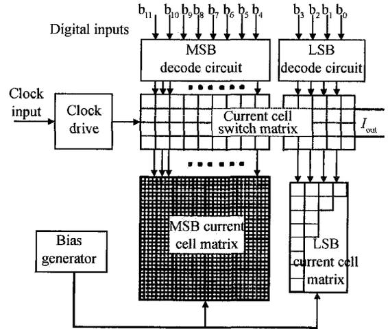
Fig. 1 Simplified DAC architecture with current
