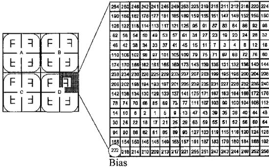
Fig. 2 Switching sequence of the  $Q^2$  random walk switching scheme
