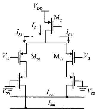
Fig. 4 Current cell with cascaded transistors
