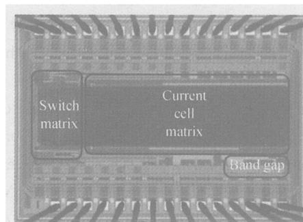
Fig. 5 Chip photograph of the D/A converter
