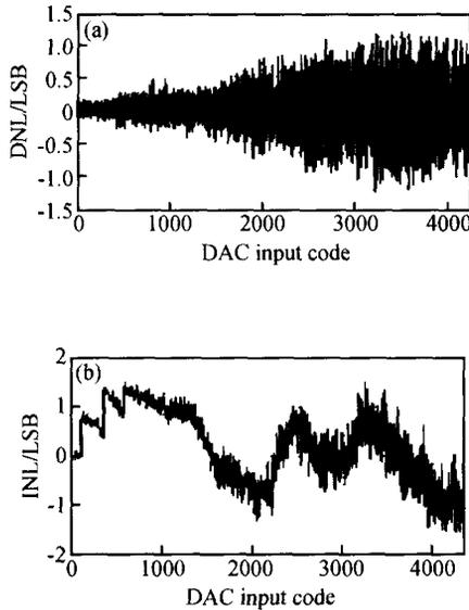
Fig. 6 DNL (a) and INL (b) measurement
