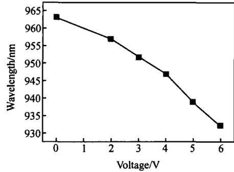
Fig. 6 Wavelength shift versus applied voltage for the device
