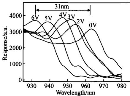
Fig. 5 Measured response spectra of the device under different tuning voltage The photodetector is biased by 3V DC.
