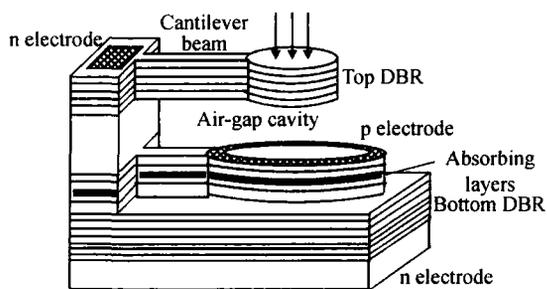
Fig. 2 Schematic structure of the MOEMS tunable RCE photodetector
