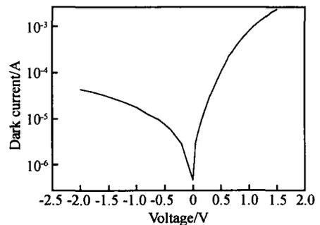
Fig. 7 Dark current of the device under different bias
