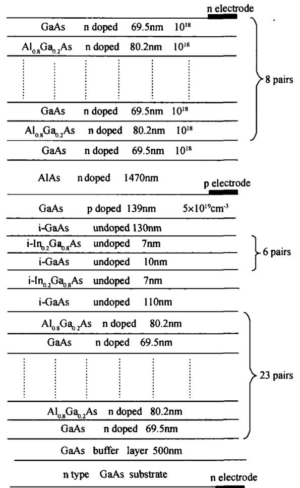
Fig. 1 Schematic diagram of epitaxial structure of the MOEMS tunable RCE photodetector
