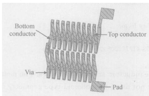
Fig. 1 Schematic diagram of a solenoid-type inductor
