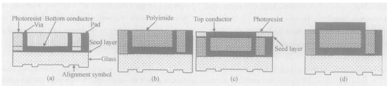
Fig. 2 Fabrication process for a complete inductor (a) Fabrication of alignment symbol, electroplating bottom conductor, via, and pad; (b) Spinning and curing polyimide, and polishing polyimide until the vias were exposed; (c) Electroplating of top conductor; (d) Removal of seed layer
