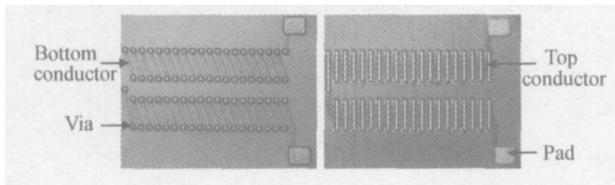
Fig. 3 SEM photos of the inductor (a) After electroplating bottom conductor ,via ,and pad; (b) A complete inductor
