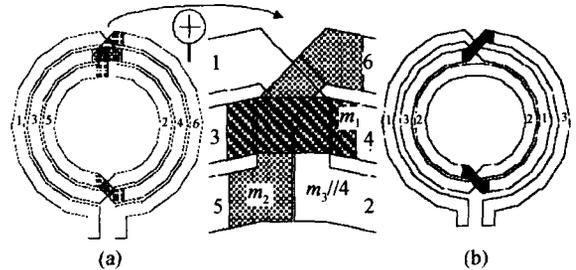
Fig. 5 Two differential inductors with low  $C_{m,m}$ . 1, 2, 3, 4, 5, and 6 are current in inductor flow direction, i. e. AC signal voltage profile. In  $m_i$ ,  $i$  represents metal layer number.
