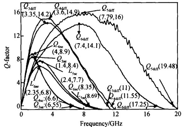
Fig. 6  $Q$  and  $f_{SR}$  of two differential inductors with low  $C_{m,m}$ .  $L_3$  is the inductor in Fig. 5 (b) and  $L_5$  is the inductor in Fig. 5 (a);  $L_4$  and  $L_6$  are the conventionally differential inductor with the same width and turns as  $L_3$  and  $L_5$ , respectively.
